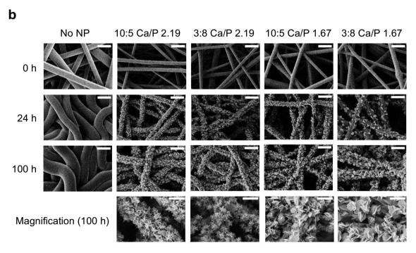
Fig. 2 (a) TEM micrographs of the fibers containing CaP NPs. Scale bar is 200 nm. (b) SEM micrographs of the fibers incubated in SBF for 24 and 100 h. Scale bar is 3  $\mu$ m, except for the magnified micrographs, where the scale bar corresponds to 1  $\mu$ m.
