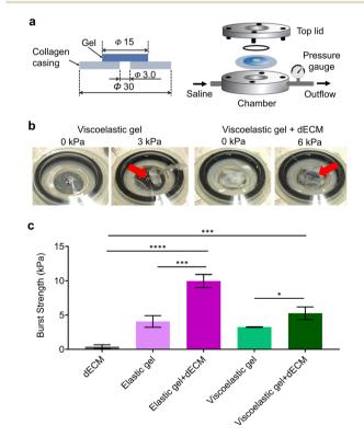
Fig. 3 Tissue-adhesive properties of gels. (a) Setup for the measurement of burst strength. (b) Macroscopic images of burst pressure measurements. (c) Burst strength of the dECM and elastic gels and viscoelastic gels with dECM microparticles (n=3). Data are presented as the mean  $\pm$  SD. \*P<0.05, \*\*\*P<0.001, and \*\*\*\*P<0.0001, analyzed using one-way ANOVA, followed by Tukey's multiple comparisons post
