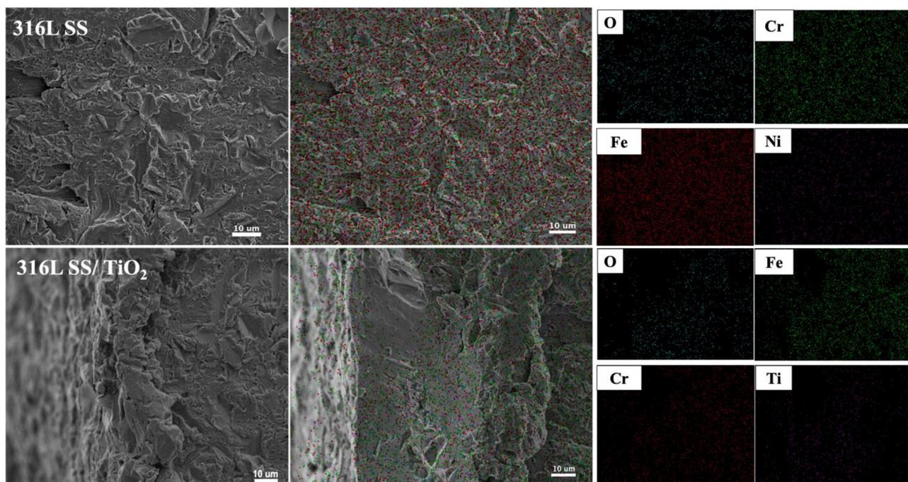
Fig. 1 SEM micrographs of 316L SS and 316L SS/TiO<sub>2</sub> surfaces. SEM micrographs reveal a rough surface because of the sandblasting. In addition to the presence of characteristic elements of SS, mapping analysis confirms the presence of Ti.
