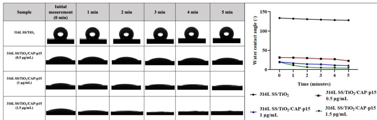
**Fig. 4** Contact angle measurement of samples (from 0–5 minutes). The adsorption of CAP-p15 contributes to a decrease in the contact angle as the concentration increases, showing values of  $31.25 \pm 2.3^\circ$  to  $22.7^\circ \pm 1.69^\circ$  for  $0.5$  µg mL<sup>-1</sup>, and  $19.85^\circ \pm 1.06^\circ$  to  $10.6^\circ \pm 1.83^\circ$ , and  $9.55^\circ \pm 0.77^\circ$  to  $3.95^\circ \pm 0.7^\circ$  for concentrations of  $0.5$ ,  $1$  and  $1.5$  µg mL<sup>-1</sup>, respectively.
