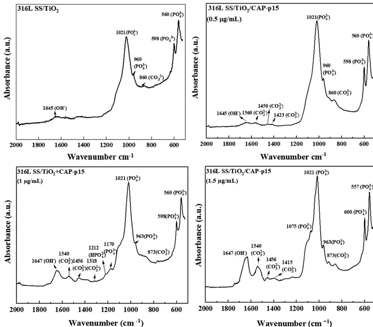
Fig. 7 ATR spectra of precipitation after 21 in AS. All samples display  $\text{PO}_4^{3-}$  groups corresponding to apatite; however, in functionalized surfaces, it is possible to observe the presence of  $\text{CO}_3^{2-}$  indicating carbonated hydroxyapatite predominantly B-type.
