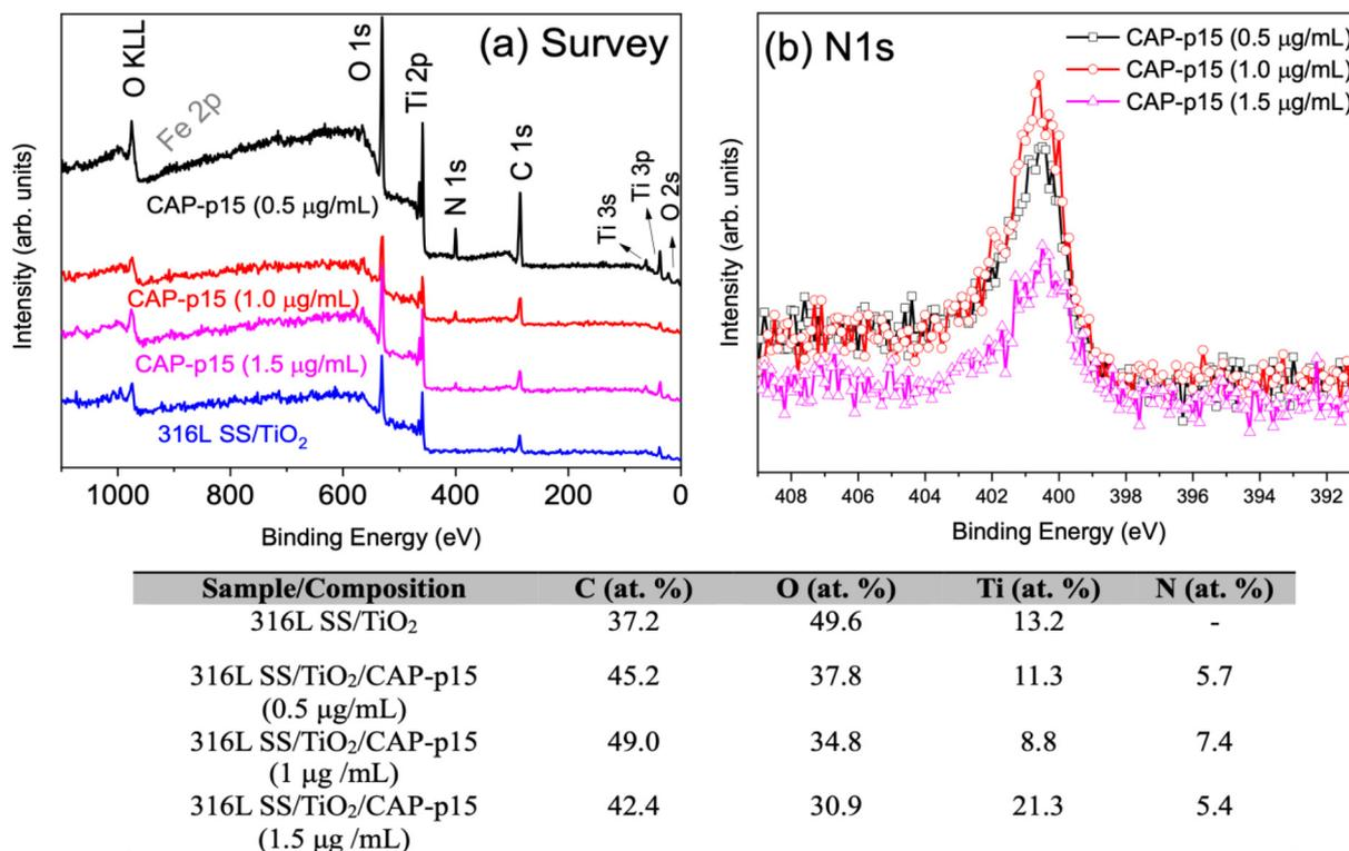
**Fig. 2** The XPS survey spectra of the pristine 316L SS/TiO<sub>2</sub> surface and after functionalization with CAP-p15 peptide at the three concentrations (a). The N content was detected for the 0.5 and 1 µg mL<sup>-1</sup> samples, while the intensity decreased for the 1.5 µg mL<sup>-1</sup> sample (b). The table reports the variation in atomic concentrations for all samples.
