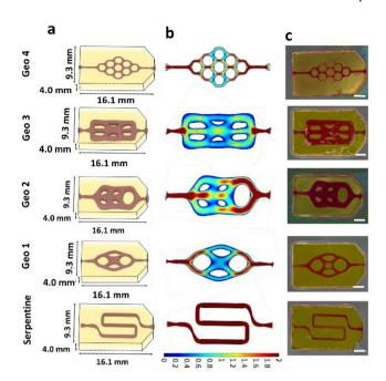
Fig. 4 Fabrication of architecture patterns for blood vessel infiltration within 3D bio-printed GelMA/PEGDA hydrogels. (a) Designed architectures in Blender with dimensions of 9.3 mm  $\times$  4 mm  $\times$  16.1 mm. (b) Fluid flow analysis images of designed architectures using COMSOL software; velocity units = mm s<sup>-1</sup>. (c) 3D bio-printed GelMA/PEGDA hydrogels perfused with red dye ink; scale bar = 2000  $\mu$ m.
