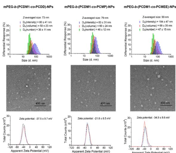
**Fig. 2** Characterization of mPEG-*b*-(PCDM1-*co*-PCDD)-NPs, mPEG-*b*-(PCDM1-*co*-PCMP)-NPs, and mPEG-*b*-(PCDM1-*co*-PCMEE)-NPs. The size distribution (top) and zeta potentials (bottom) of NPs were measured by DLS, and their morphology (middle) was imaged by TEM.
