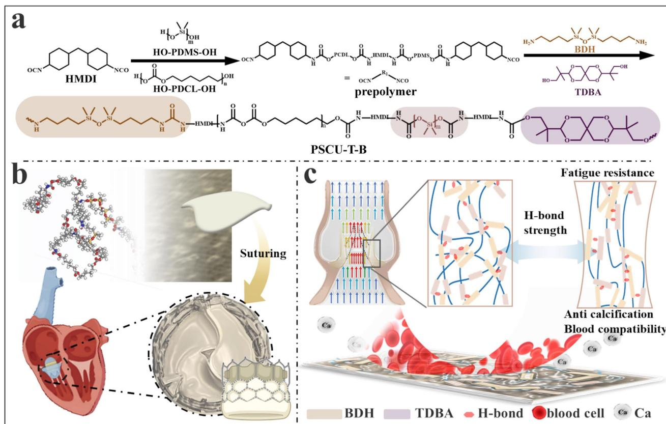
**Fig. 7** Design and synthesis of polyurethane with enhanced fatigue resistance, anti-calcification and blood compatibility for heart valves. (a) Structure of polyurethane. (b) Processing of artificial heart valves. (c) Polyurethane heart valves having fatigue resistance, anti-calcification, and blood compatibility. Reproduced from ref. 86 with permission. Copyright 2024, Elsevier.
