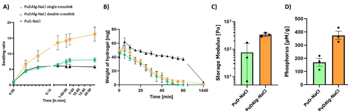
Fig. 7 (A) Swelling ratios during 24 h for PuD-NaCl; PuDAlg-NaCl crosslink with only STMP; and PuDAlg-NaCl STMP + CaCl<sub>2</sub> double crosslink. (B) Enzymatic degradation of the same three formulations for 24 h. (C and D) Structural properties of PuD-NaCl and PuDAlg-NaCl: evaluation of elastic modulus and phosphorus contents.
