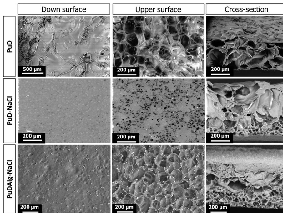
**Fig. 3** Scanning electron microscopy of PuD, PuD-NaCl and PuDAlg-NaCl. Images highlighted with the absence or presence of porosities from down and upper surfaces and cross-sections. White dots on PuDAlg-NaCl membranes correspond to calcium ions. Gradient of pore sizes is visible on PuD-NaCl and PuDAlg-NaCl.
