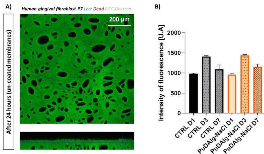
**Fig. 9** (A) Barrier effect observed by confocal analysis at day 1 performed with human gingival fibroblasts seeded on the smooth surface. Absence of cells inside pores indicated that no infiltration nor migration has occurred. (B) Indirect cell viability on PuDALg-NaCl up to 7 days.
