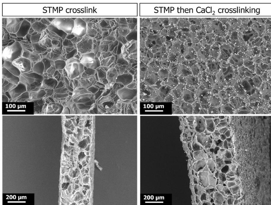
Fig. 4 SEM observations on PuDAlg-NaCl with and without  $\text{CaCl}_2$  cross-linking.
