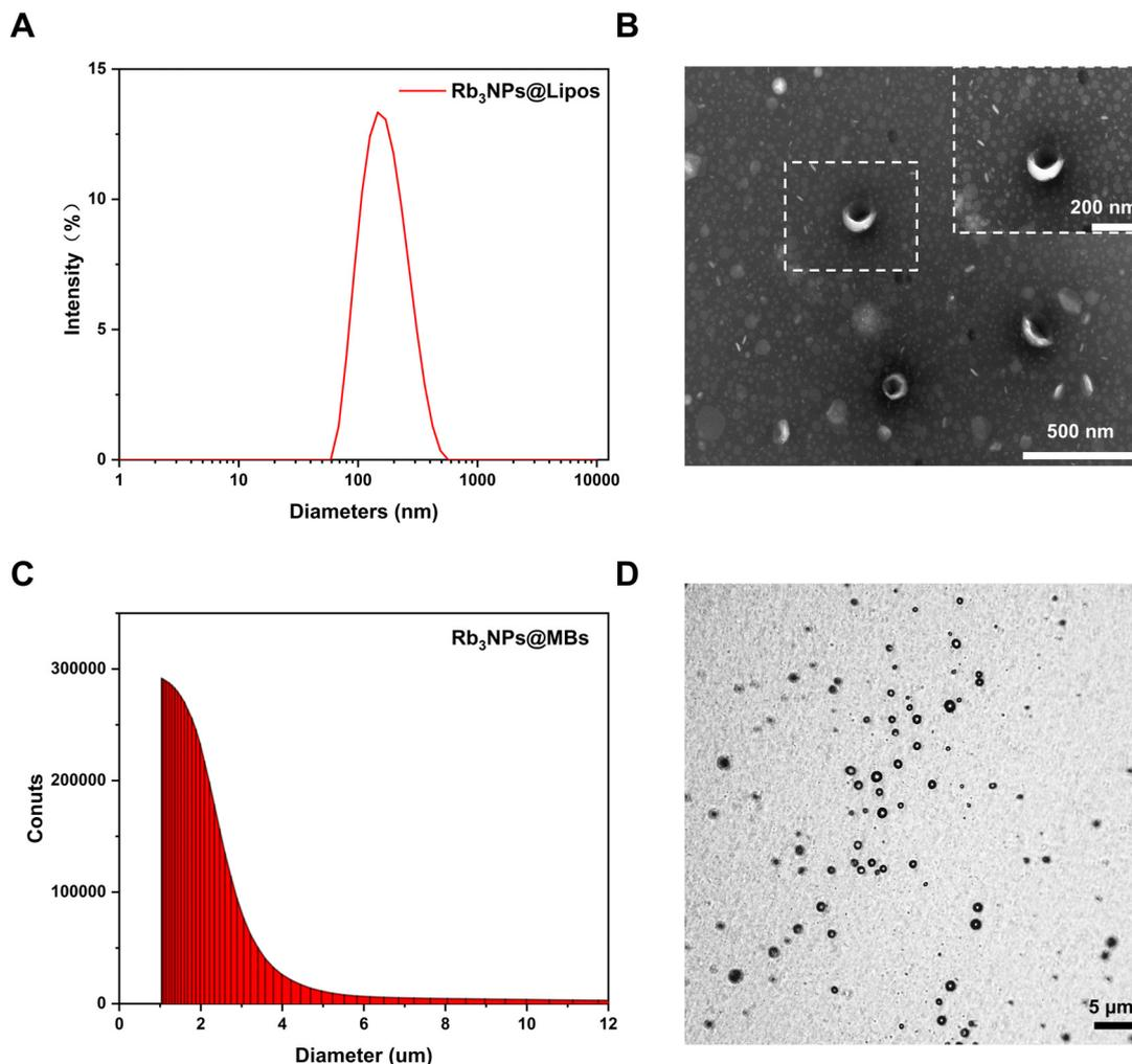
**Fig. 1** The characterization of Rb<sub>3</sub>NPs@Lipos and Rb<sub>3</sub>NPs@MBs. (A) The particle size of Rb<sub>3</sub>NPs@Lipos was measured by DLS. (B) The morphological structure of Rb<sub>3</sub>NPs@Lipos was observed by TEM. (C) The concentration and size distribution of Rb<sub>3</sub>NPs@MBs were measured by PSS. (D) The structures of Rb<sub>3</sub>NPs@MBs were observed light microscope.
