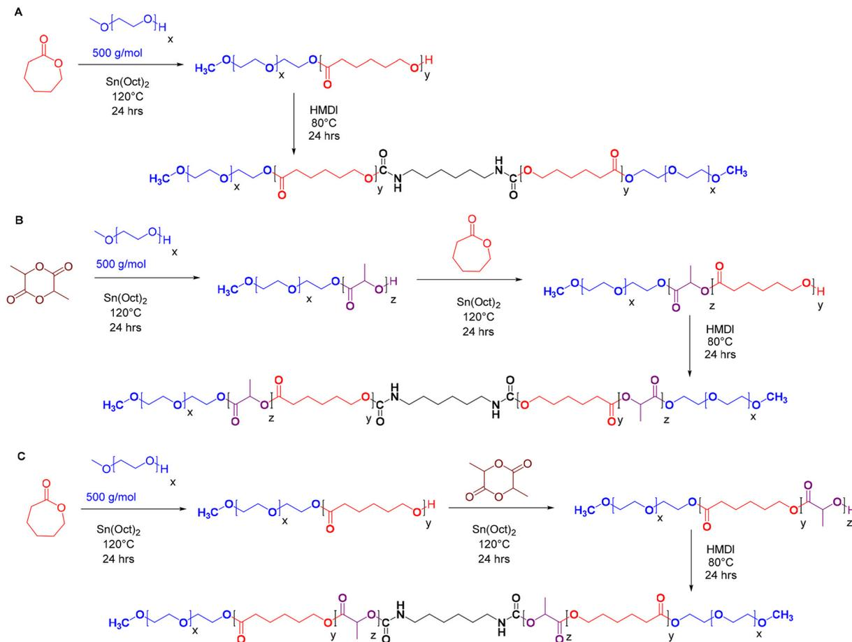
**Scheme 1** Polymer synthesis. Schematic representation of the synthetic procedures followed to prepare: (A) PECE triblock co-polymer; (B) mPEG-*b*-PLA-*b*-PCL-HMDI-PCL-*b*-PLA-mPEG pentablock co-polymer (PELCLE); and (C) mPEG-*b*-PCL-*b*-PLA-HMDI-PLA-*b*-PCL-mPEG pentablock co-polymer (PECLCE).
