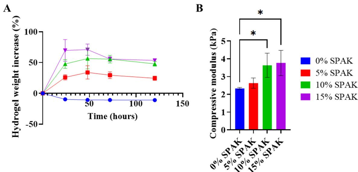
**Fig. 1** Characterisation of swelling and compressive modulus in UV cast SPAK-PEGDA hydrogels. (A) 5 Day *in vitro* swelling of 10% 575 Da PEGDA hydrogels containing 0%–15% SPAK. (B) Compressive modulus of swollen SPAK-PEGDA hydrogels. Values presented as mean  $\pm$  standard deviation ( $n = 3$ ). \* denotes a statistical difference with  $P \leq 0.05$  determined by 1 way ANOVA with Tukey's *post hoc* multiple comparisons.
