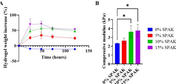
Fig. 1 Characterisation of swelling and compressive modulus in UV cast SPAK-PEGDA hydrogels. (A) 5 Day *in vitro* swelling of 10% 575 Da PEGDA hydrogels containing 0%–15% SPAK. (B) Compressive modulus of swollen SPAK-PEGDA hydrogels. Values presented as mean  $\pm$  standard deviation (n = 3). \* denotes a statistical difference with  $P \le 0.05$  determined by 1 way ANOVA with Tukey's *post hoc* multiple comparisons.
