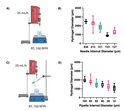
Fig. 6 Development of alginate bead encapsulation system. (A) Schematic of alginate bead production with dropwise release from a needle. (B) Effect of needle internal diameter on alginate bead size (n = 20 beads per condition, central line = median, box = upper and lower quartiles). (C) Schematic of alginate bead production with dropwise release from a pulled glass pipette. (D) Effect of pipette internal diameter on alginate bead size (n = 10 beads per condition).
