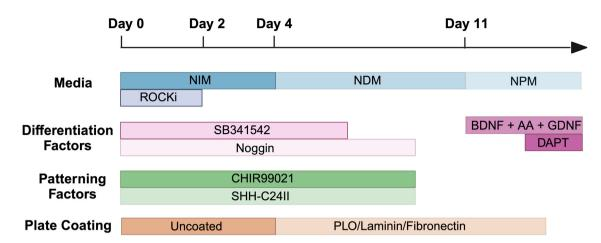
Scheme 1 Schematic of differentiation methodology from hiPSCs to dopaminergic neurons, adapted from Kirkeby et al.<sup>7,8</sup> Abbreviations include neural induction media (NIM), neural differentiation media (NDM), neural proliferation media (NPM), ROCK inhibitor (ROCKi), brain-derived neurotrophic factor (BDNF), ascorbic acid (AA), glial cell line-derived neurotrophic factor (GDNF), poly-L-ornithine (PLO).
