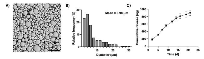
Fig. 4 Synthesis and characterisation of tacrolimus-loaded microparticles. (A) Scanning electron micrograph of tacrolimus-loaded microparticles, scale bar =  $30 \mu m$ . (B) Frequency distribution of microparticle diameter from scanning electron micrographs (n = 3 images,  $\sim 90$  measurements per image). (C) Cumulative release of tacrolimus per mg of microparticles over three weeks (n = 3 samples  $\pm$  SD).
