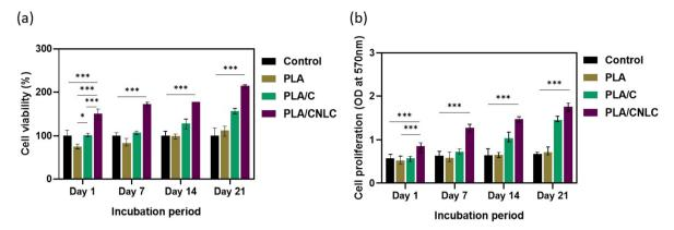
Fig. 7 Cell viability percentage and growth rate for 3D printed PLA, PLA/C, and PLA/CNLC scaffolds using MTT assay. (a) Viability percentage (%) vs. incubation period and (b) OD at 570 nm vs. incubation period. The data are presented as mean  $\pm$  S.D. for n = 3. \*\* indicates significance for p < 0.01and \*\*\* indicates p < 0.001.
