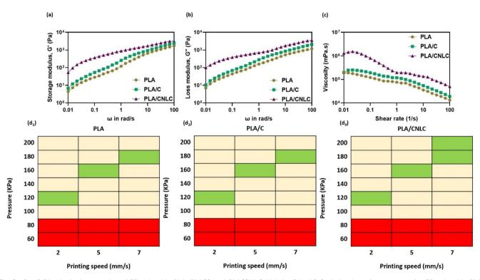
Fig. 2 (a-c) Rheological properties of 3D printable PLA, PLA/C and PLA/CNLC bioinks. (d<sub>1</sub>-d<sub>3</sub>) Optimization of parameters for 3D printable PLA, PLA/C and PLA/CNLC bioinks.
