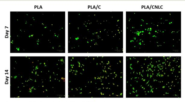
Fig. 8 Live/dead staining of 3 T3 cells seeded on PLA, PLA/C, and PLA/CNLC scaffolds for varying culture time durations.
