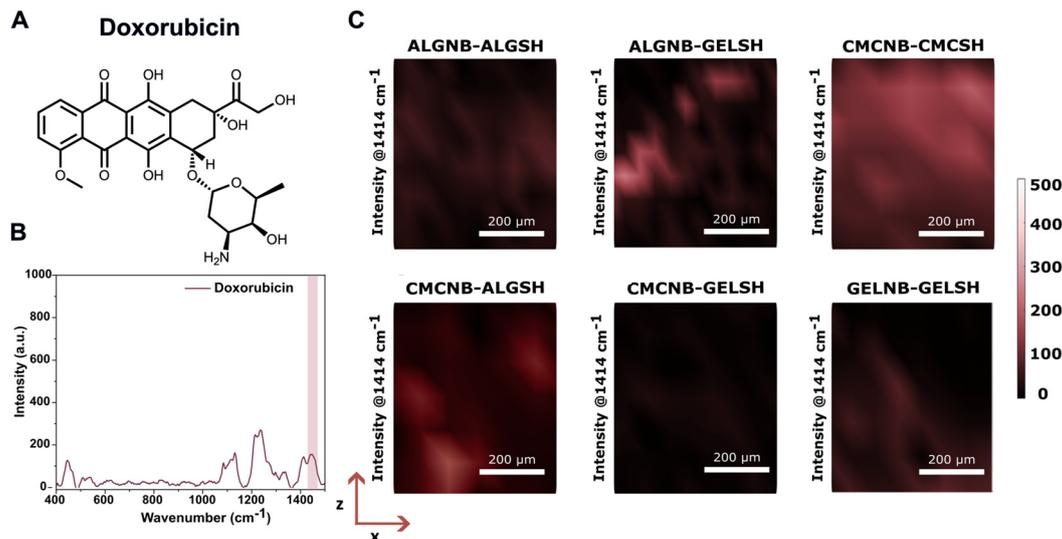
**Fig. 6** (A) Chemical structure of doxorubicin (DOXO). (B) SERS spectrum of doxorubicin showing its main vibrational peaks. (C) SERS intensity maps for DOXO across hydrogels with different compositions. The intensity at 1414 cm<sup>-1</sup> is represented across the xz directions for each gel.
