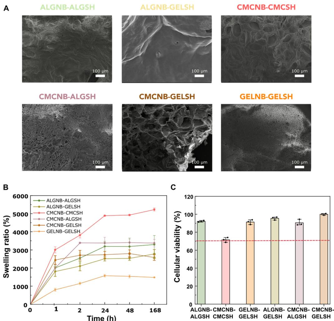
**Fig. 4** Characterization of the hydrogels formed through thiol-ene crosslinking at 3% (w/v) concentration of the highest functionalized polymer. (A) SEM images of the freeze-dried hydrogels. (B) Swelling ratio of all combinations of hydrogels measured at different time points over a week of incubation at 37 °C. (C) Biocompatibility of the hydrogels.
