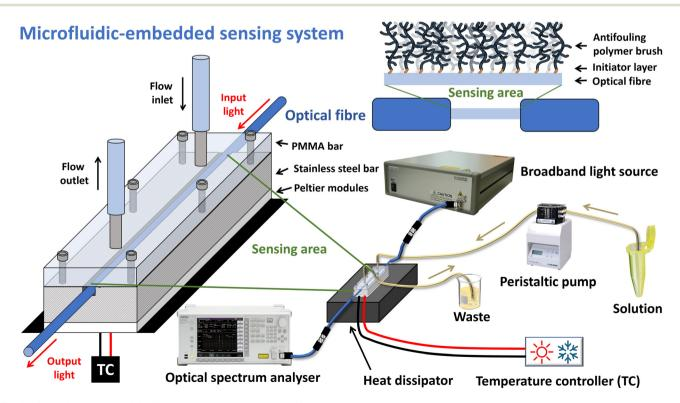
Fig. 1 General schematic of the fibre-optic sensing system used herein.
