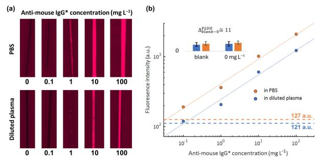
Fig. 4 (a) Fluorescence microscopy images of LPG fibres exposed to increasing concentrations of anti-mouse IgG\* in PBS (top row) and in diluted plasma (bottom row); (b) dependence of fluorescence intensity on anti-mouse IgG\* concentration measured on ATB-coated LPG fibres in PBS (orange) and in 10% human blood plasma diluted in PBS (blue).
