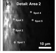
Fig. 2 (a) SEM image of a bare optical fibre; (b) SEM image of an ATB-coated LPG fibre with selected areas for EDS analysis: area 1 shows very smooth surface and pertains to an area of the fibre where the polymerization did not run properly, whereas area 2 confirms the presence of terpolymer nano-brush; (c) enlarged SEM image of area 2 of the ATB-coated LPG fibre with 5 selected spots for EDS analysis.
