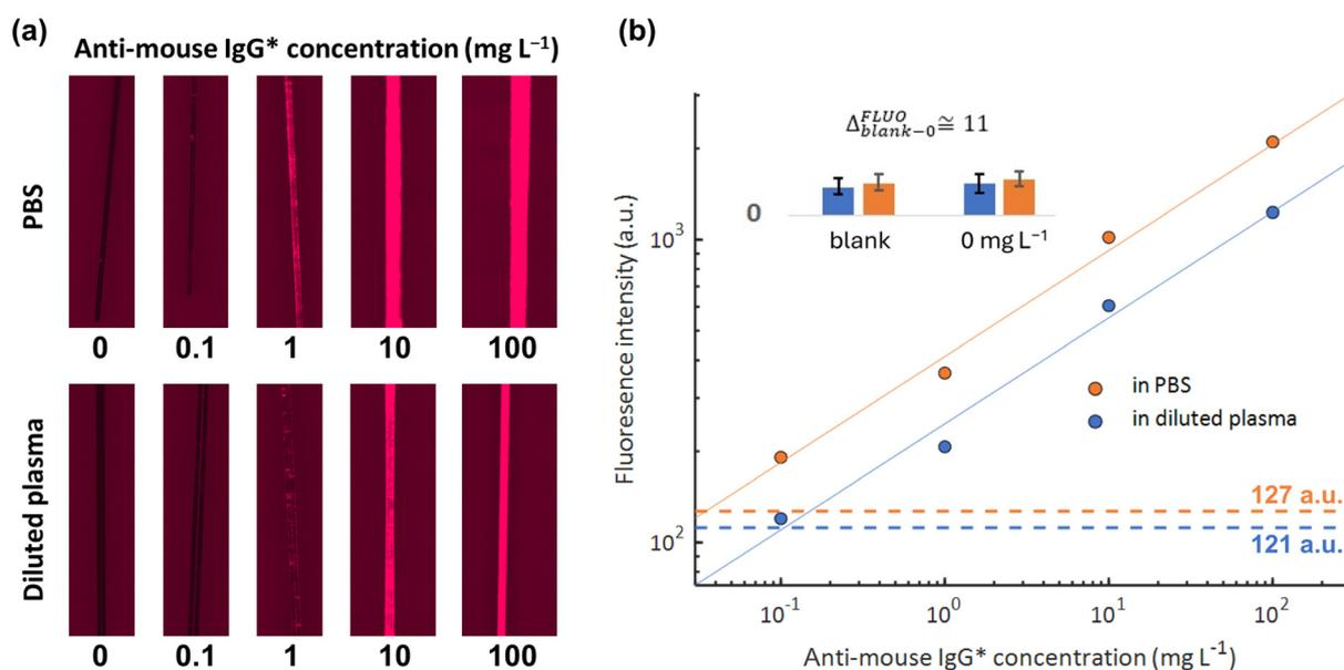
Fig. 4 (a) Fluorescence microscopy images of LPG fibres exposed to increasing concentrations of anti-mouse IgG\* in PBS (top row) and in diluted plasma (bottom row); (b) dependence of fluorescence intensity on anti-mouse IgG\* concentration measured on ATB-coated LPG fibres in PBS (orange) and in 10% human blood plasma diluted in PBS (blue).
