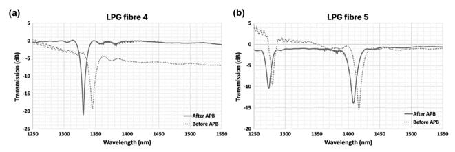
Fig. 3 Transmission spectra of optical fibres (measured in air): LPG fibre 4 (a) and LPG fibre 5 (b) before (dotted grey curve) and after (grey curve) the deposition of ATB coatings.
