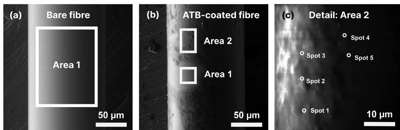
**Fig. 2** (a) SEM image of a bare optical fibre; (b) SEM image of an ATB-coated LPG fibre with selected areas for EDS analysis: area 1 shows very smooth surface and pertains to an area of the fibre where the polymerization did not run properly, whereas area 2 confirms the presence of terpolymer nano-brush; (c) enlarged SEM image of area 2 of the ATB-coated LPG fibre with 5 selected spots for EDS analysis.
