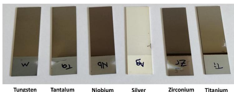
**Fig. 2** PVD coatings with different metals.
