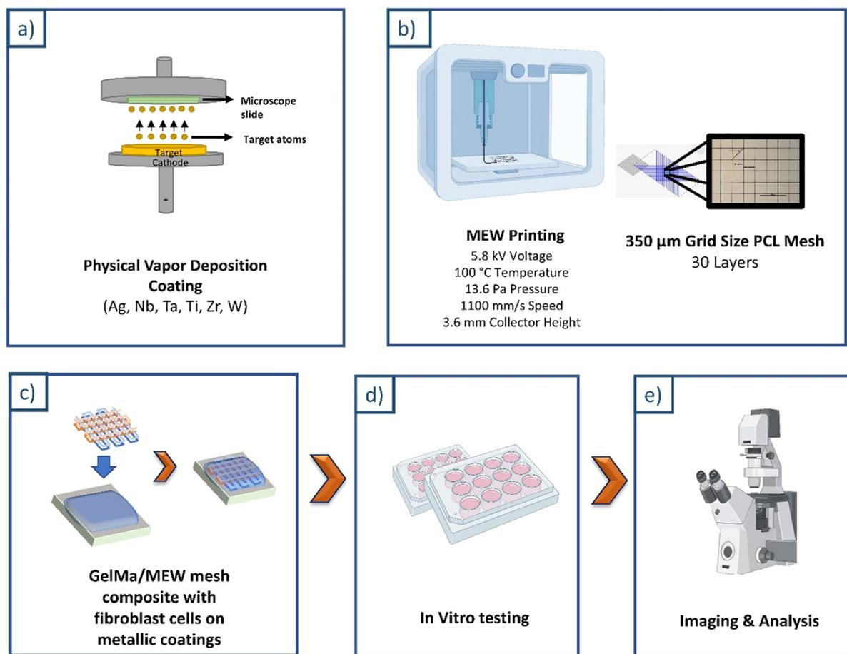
**Fig. 1** Steps of the study. (a) PVD metallic coatings of the slides; (b) PCL mesh printing using MEW; (c) placement of the GelMa/MEW mesh composite scaffold containing fibroblasts on coated slides; (d) *in vitro* testing; and (e) imaging and analysis of samples.
