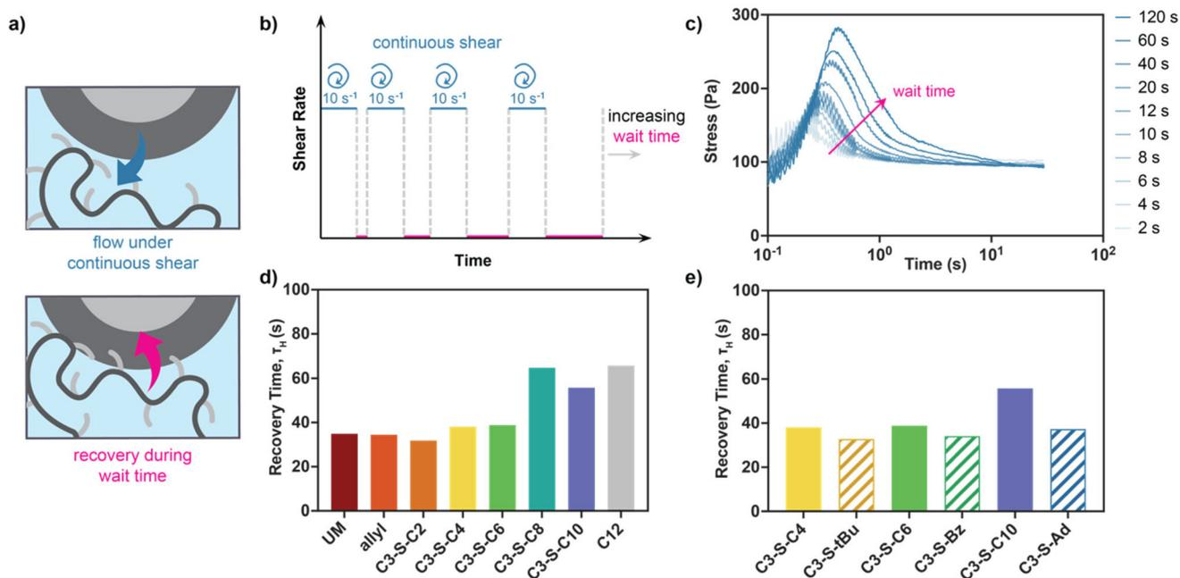
**Fig. 4** Recovery properties of PNP library. (a) Simplified depiction of polymer–nanoparticle interaction under flow and wait time conditions. (b) Diagram describing experimental protocol to determine recovery times. (c) Representative stress overshoot measurement of a C3-S-Ad PNP hydrogel with increasing wait times. Recovery times,  $\tau_r$ , of (d) linear and (e) steric/pi stacking PNP derivatives determined by fitting stress overshoots.
