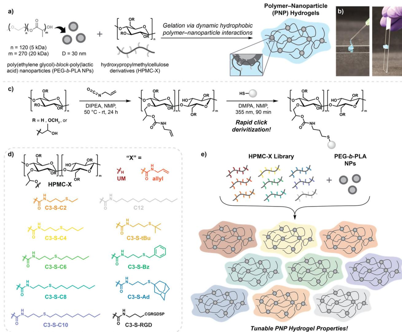
**Fig. 1** Preparation of PNP hydrogel library. (a) General schematic of PNP hydrogel preparation. (b) Photographs demonstrating injectability and recovery of PNP hydrogels. Blue color corresponds to a dye used for visualization only. (c) Synthetic scheme to prepare HPMC-X derivatives. (d) Library of HPMC-X derivatives prepared. (e) Schematic depiction of PNP hydrogel library preparation.
