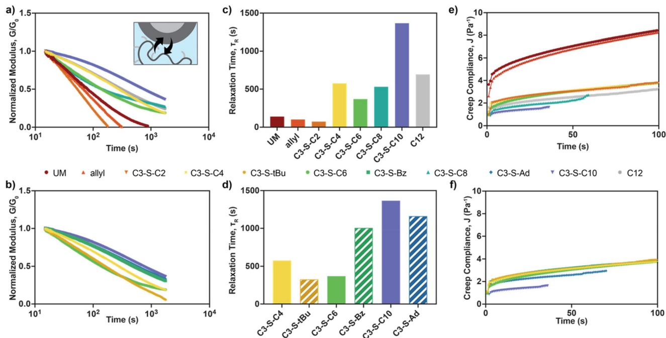
**Fig. 3** Dynamic properties of PNP library. Stress relaxation measurements of (a) linear and (b) steric/pi stacking PNP derivatives (5% strain). Relaxation times,  $\tau_R$ , of (c) linear and (d) steric/pi stacking PNP derivatives determined from fitting of relaxation curves in (a) and (b). Creep compliance of (e) linear and (f) steric/pi stacking PNP derivatives under a constant applied stress of 20 Pa.
