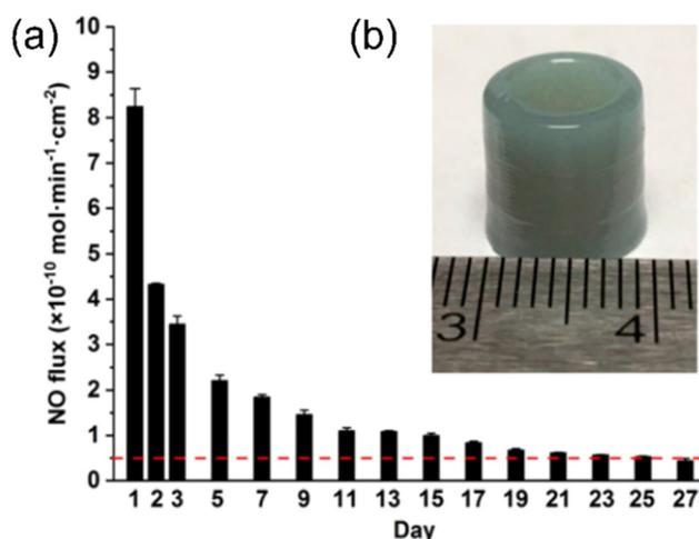
**Fig. 8** (a) NO release from SNAP-doped silicone rubber tube with PDMS construct in PBS solution at 37 °C. (b) Picture of the 3D-printed SNAP-loaded construct with PDMS coating. Reprinted (adapted) with permission from W. Li, Y. Yang, C. J. Ehrhardt, N. Lewinski, D. Gascoyne, G. Lucas, H. Zhao and X. Wang, *ACS Appl. Bio Mater.*, 2021, 4, 7653–7662. Copyright 2021.
