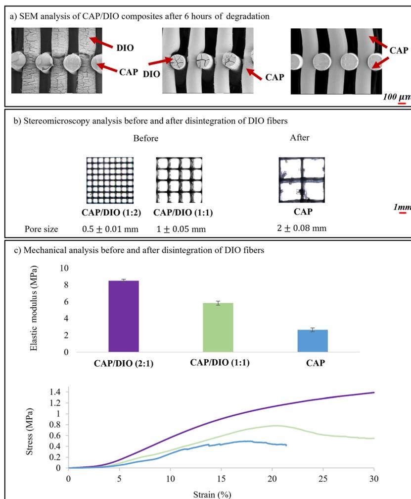
**Fig. 4** *In vitro* degradation of DIO/CAP under acidic conditions. (a) Morphological study conducted via SEM analysis ( $n = 3$ ). (b) Stereomicroscopy images of the composites before and after degradation to calculate the pore size ( $n = 5$ ). (c) Changes in mechanical response and elastic modulus of the composites under compression ( $n = 5$ ).
