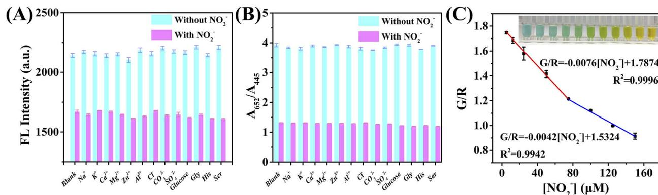
Fig. 6 Selectivity and anti-interference performance of the dual-mode sensor (interferent concentration: 100  $\mu\text{M}$  each): (A) fluorescence response and (B) colorimetric response. (C) Linear relationship between G/R and  $\text{NO}_2^-$  concentration (Inset: Photograph of the colorimetric sensing system in the presence of  $\text{NO}_2^-$  at increasing concentrations from left to right: 0, 2.5, 5, 12.5, 25, 50, 75, 100, 125, 150, and 175  $\mu\text{M}$ ).
