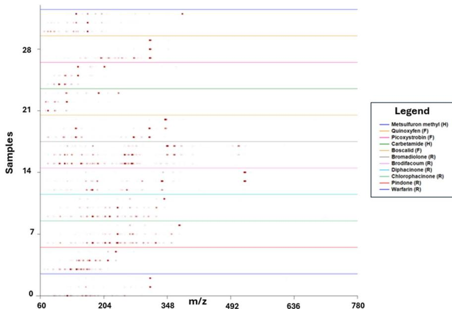
Fig. 2 Heat map of rodenticide (R), fungicide (F) and herbicide (H) reference standards ( $1000 \text{ mg L}^{-1}$ , with the exception of brodifacoum at  $50 \text{ mg L}^{-1}$ ) at low (30 V), medium (60 V) and high (90 V) voltages, from top to bottom respectively. Heat map was generated by Mass Mountaineer™ software (Ver. 7.1.25).
