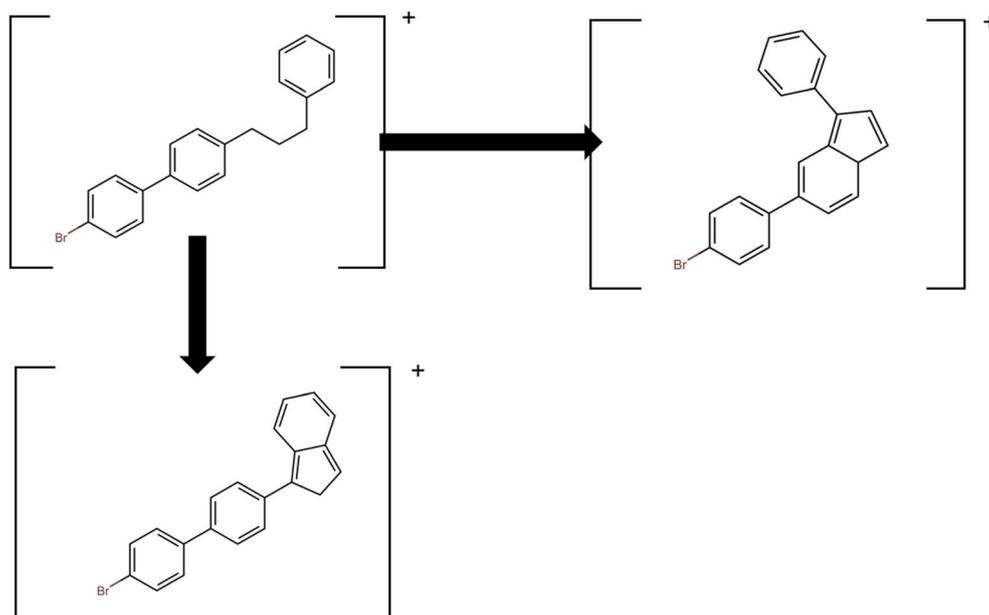
**Fig. 4** Suspected bromadiolone fragments. The existing fragment (top left) is suspected to cyclize in two proposed ways (right and bottom) while retaining a detectable positive ion charge.
