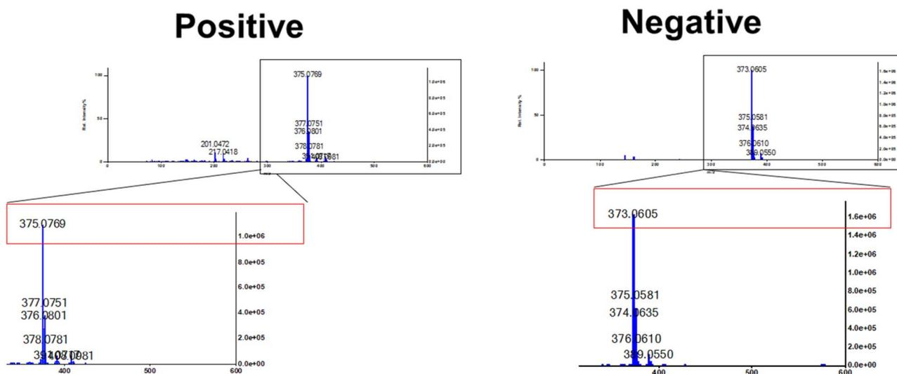
**Fig. 7** Sample comparison of positive (left) and negative (right) mode on DART-ToF to analyze 100 mg L<sup>–1</sup> chlorophacinone. The red box highlights signal intensity of the base peak between both modes.
