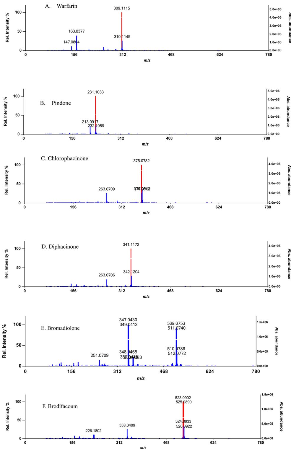
Fig. 3 Mass spectra of rodenticides at 1000 mg L<sup>-1</sup> (A) warfarin, (B) pindone, (C) chlorphacinone, (D) diphacinone, (E) bromadiolone and 50 mg L<sup>-1</sup> (F) brodifacoum and collected by DART-ToF MS in positive ion mode at +30 V with the glass capillary background subtracted. Data was visualized from a centroided text file using Mass Mountaineer™, where relative intensities were mapped against m/z. The red peak indicates the m/z used for protonated molecule comparisons.
