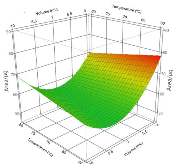
Fig. 4 Three-dimensional response surface plot illustrating the combined effect of sample volume and extraction temperature on the analytical response (Area per  $\mu\text{g}$ ) obtained by HS-GC-FID, with the equilibration time fixed at 25 min.
