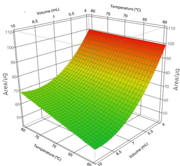
Fig. 2 Response surface plot showing the effect of sample volume and extraction temperature on HS-GC-FID response (Area per  $\mu\text{g}$ ), with equilibration time fixed at 15 min. The plot indicates that lower sample volumes combined with higher extraction temperatures enhance headspace partitioning efficiency and yield higher analytical responses.
