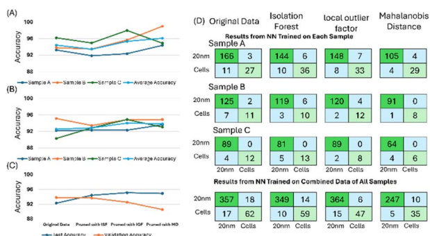
Fig. 4 Cells vs. (cells with all 20 nm CD66b as one class for each sample). (A) Test accuracies for averaged and individual samples. (B) Validation accuracies for averaged and individual samples. (C) Cells vs. (cells with all 20 nm CD66b as one class combined data) test/validation accuracy. (D) Confusion matrices for each sample plotted before and after application of the outlier removal methods.
