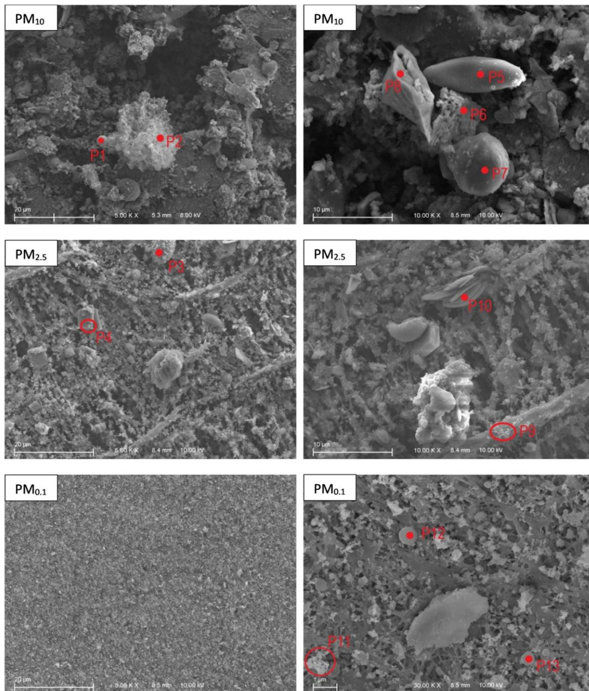
Fig. 2 SEM imaging of PM<sub>10</sub> (left at 5000× magnification; right at 10 000× magnification), PM<sub>2.5</sub> (left at 5000× magnification; right at 10 000× magnification) and PM<sub>0.1</sub> (left at 5000× magnification; right at 30 000× magnification).
