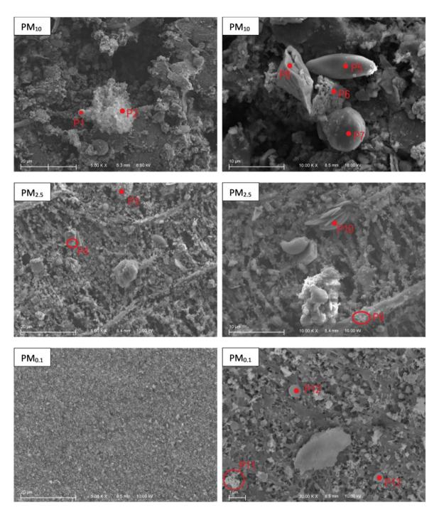
Fig. 2 SEM imaging of  $PM_{10}$  (left at  $5000 \times$  magnification; right at  $10\,000 \times$  magnification),  $PM_{2.5}$  (left at  $5000 \times$  magnification; right at  $10\,000 \times$  magnification) and  $PM_{0.1}$  (left at  $5000 \times$  magnification; right at  $30\,000 \times$  magnification).
