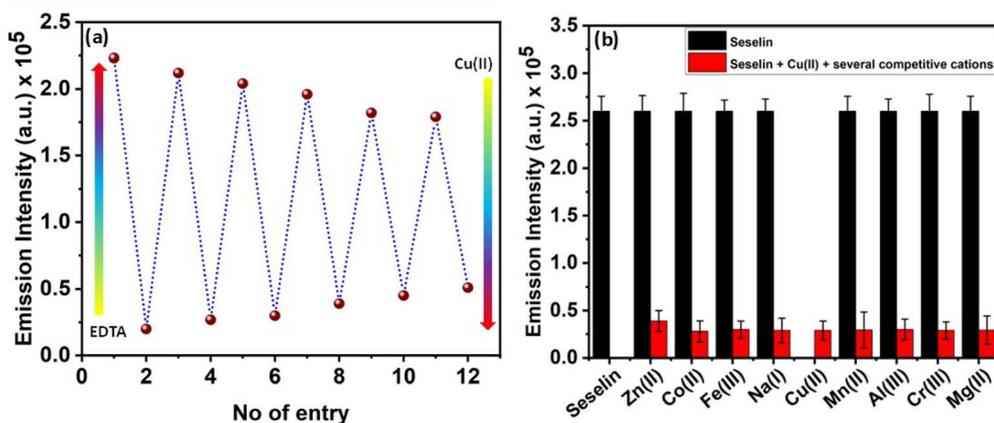
Fig. 3 (a) Reversibility experiment of SS by alternate addition of Cu(II) and EDTA in MeOH– $\text{H}_2\text{O}$  (7 : 3 v/v) HEPES buffer solution. (b) Change in emission intensity of the SS–Cu(II) conjugate in the presence of several competitive cations in MeOH– $\text{H}_2\text{O}$  (7 : 3 v/v) HEPES buffer solution.
