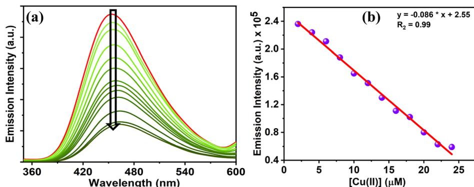
Fig. 2 (a) Change in emission intensity of SS ( $5 \times 10^{-6}$  M) after incremental addition of Cu(II) (1–25  $\mu$ M) in MeOH–H<sub>2</sub>O (7 : 3 v/v) HEPES buffer solution at pH 7.4. (b) Determination of the LOD value of SS for Cu(II) ions.
