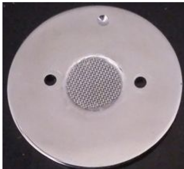
Fig. 1 Photograph of the button sample holder.
