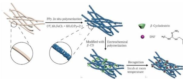
Fig. 8 Illustrates the synthesis and electrochemical detection of dinotefuran using PCL/PPy/ $\beta$ -CD flexible sensor.<sup>128</sup>
