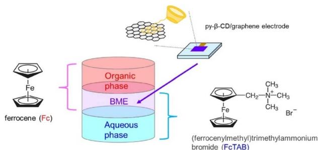
Fig. 5 Concept of Fc analysis in bicontinuous microemulsions using py- $\beta$ -CD modified monolayer graphene electrode.<sup>95</sup>
