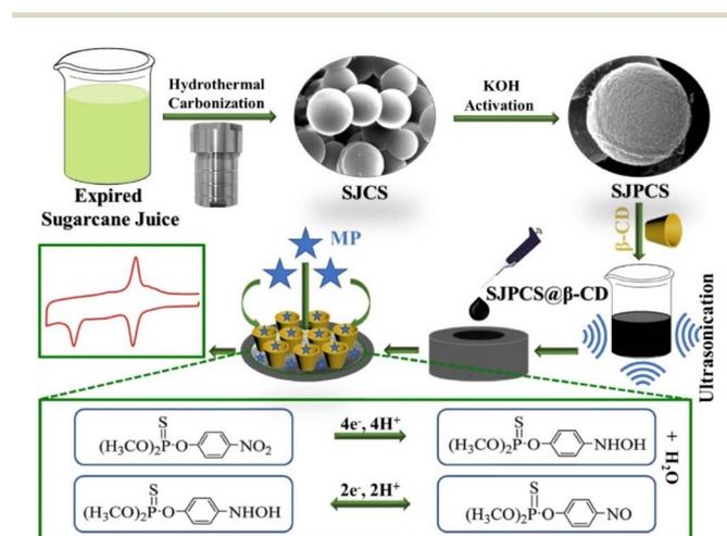
Fig. 12 Determination of MP using electrochemical sensor fabricated from  $\beta$ -CD (SJPCS@ $\beta$ -CD).<sup>149</sup>
