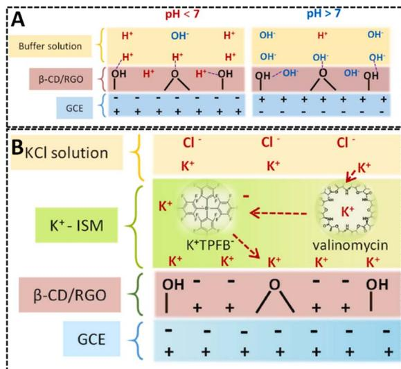
Fig. 7 (A) Representations for pH response mechanism of  $\beta$ -CD/RGO/GCE and (B) representations for  $K^+$  response mechanism of  $K^+$ -ISM/ $\beta$ -CD/RGO/GCE.<sup>121</sup>
