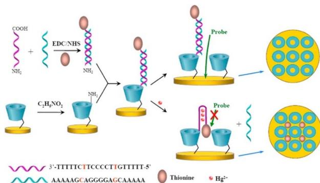
**Fig. 11** Schematic of the electrochemical sensor for detecting  $\text{Hg}^{2+}$ .<sup>147</sup>
