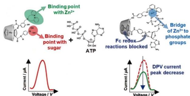
Fig. 3 The *cis*-diol binding of ribose with PBA causes a reduction of DPV current peak as the Fc redox reaction is blocked.<sup>51</sup>
