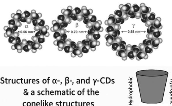
Fig. 2 Schematic representation of the molecular structures and cavity dimensions of  $\alpha$ -,  $\beta$ -, and  $\gamma$ -CDs, each comprising 6, 7, and 8 glucopyranose units, respectively. The conelike illustrations depict their truncated cone geometry with a hydrophobic inner cavity and hydrophilic exterior, which underlies their ability to form host-guest inclusion complexes in electrochemical sensing applications.
