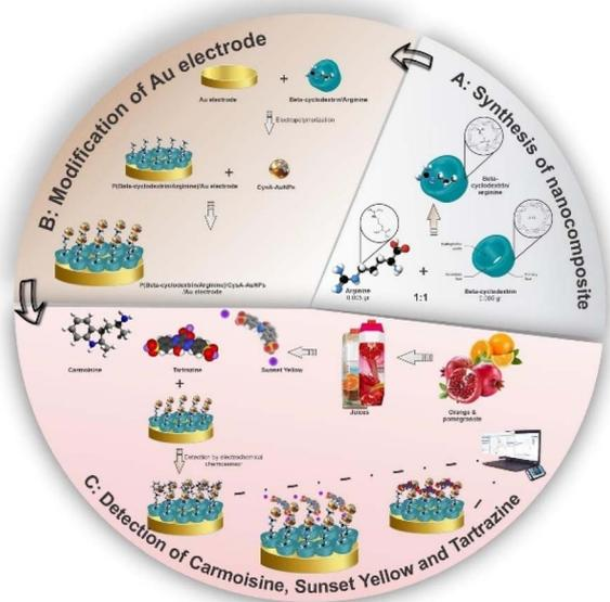
Fig. 10 Schematic illustration of the chemosensor (P( $\beta$ -CD/Arg)/CysA–AuNPs/AuE) fabrication process for detection of carmoisine, sunset yellow, and tartrazine in juices.<sup>133</sup>
