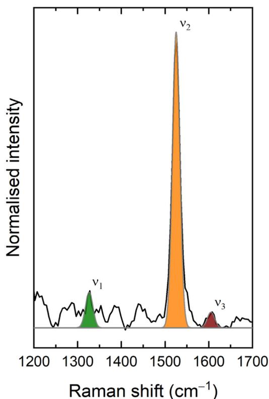
Fig. 2 For each spectrum, peak fitting has been performed. The vibration at 1326 cm<sup>-1</sup> ( $v_1$ ) has been chosen to represent the chlorophyll content and the band at 1525 cm<sup>-1</sup> ( $v_2$ ) describes the carotenoid content, while the polyphenol content is indicated by the peak at 1604 cm<sup>-1</sup> ( $v_3$ ).
