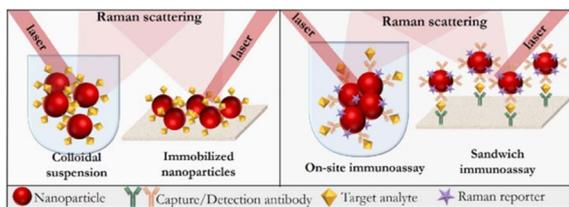
Fig. 2 Schematic representation of the direct and indirect approaches for SERS-based detection.<sup>87</sup>
