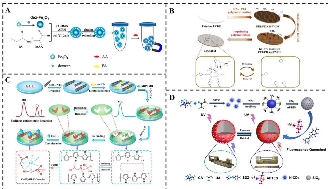
Fig. 14 (A) Schematic illustration of the process for preparation of dex-MMIPs.<sup>176</sup> (B) Schematic illustration of constructing LINMIMs for selective recognition and separation of lincomycin.<sup>177</sup> (C) Schematic diagram of MIP/MWCNTs-Au/GCE for GLY indirect determination, in which the Cu(II)-GLY complex is well formed.<sup>178</sup> (D) Schematic diagram of the MIP preparation process.<sup>179</sup>
