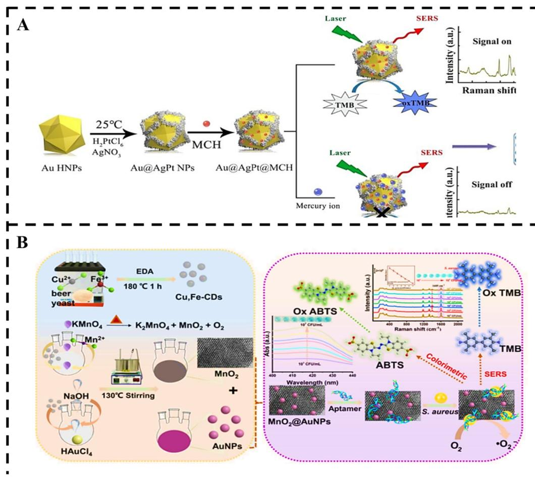
Fig. 10 (A) Schematic illustration of the preparation of Au@AgPt@MCH and the colorimetric/SERS sensing strategy for Hg<sup>2+</sup>.<sup>129</sup> (B) Schematic diagram of MnO<sub>2</sub>@AuNP synthesis and the mechanism of specific *S. aureus* detection.<sup>130</sup>
