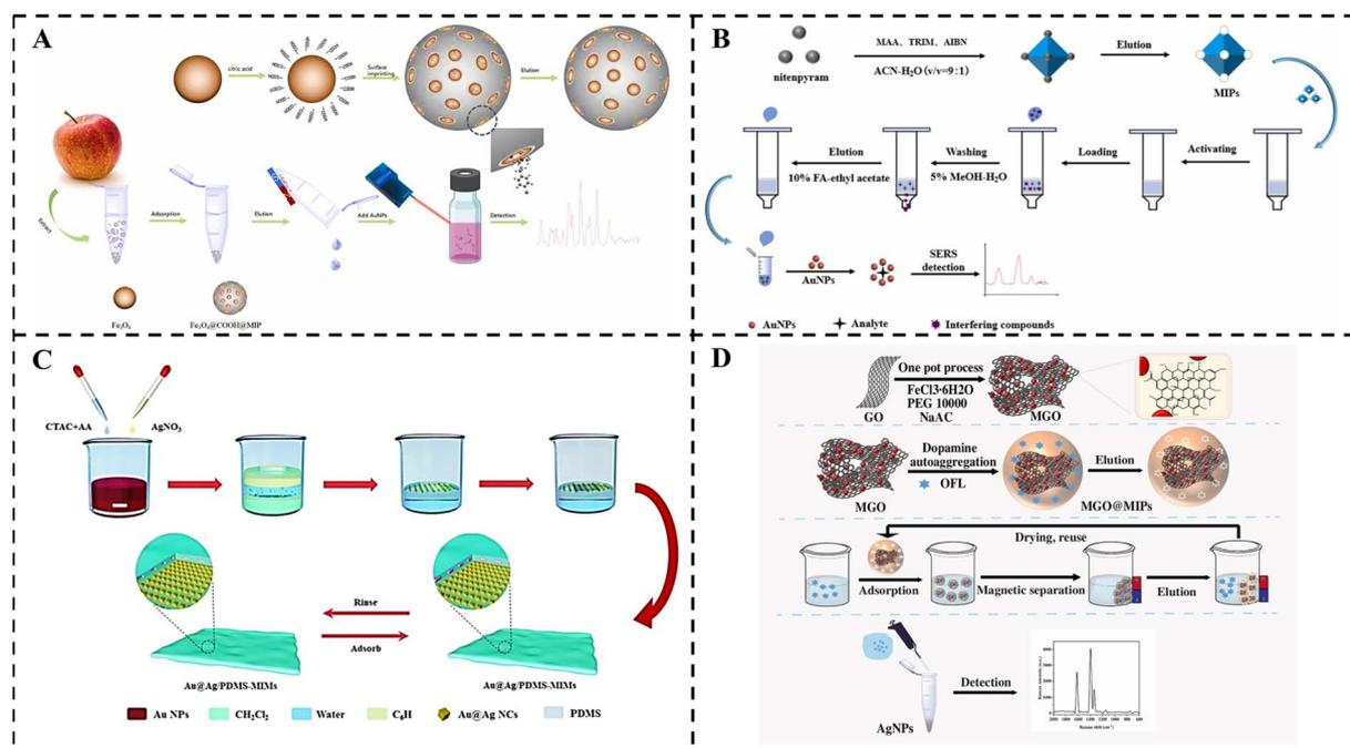
Fig. 16 (A) Analysis of myclobutanil and tebuconazole in apple by a novel SERS method based on MMIP-SERS.<sup>188</sup> (B) Schematic of the preparation process of imprinted polymers and MIPs-SERS for extracting and detecting nitenpyram.<sup>189</sup> (C) The synthesis and SERS detection process of AAP-MIMs.<sup>190</sup> (D) Schematic illustration for the preparation process of MGO@MIP particles and their application in ofloxacin detection using SERS signals.<sup>191</sup>
