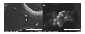
Fig. 3 SEM images of (A) the BiP-Am sample at 100  $\mu$ m scale and (B) the BiP-Am-nicotine aggregate at 30  $\mu$ m scale.
