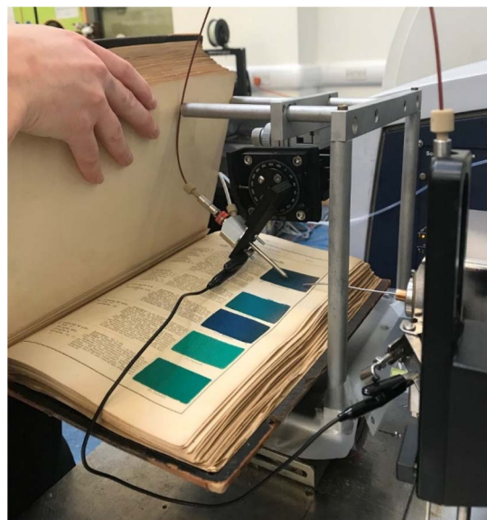
Fig. 4 DESI-MS set-up for sampling of historical dye samples. Reproduced from ref. 12 under CC-BY 4.0 license conditions† doi: https://doi.org/10.1021/acs.analchem.2c03281 .
