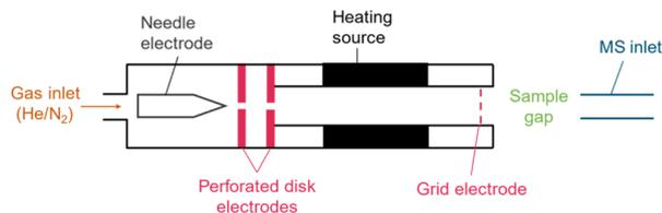
Fig. 2 Schematic representation of a DART-MS source.
