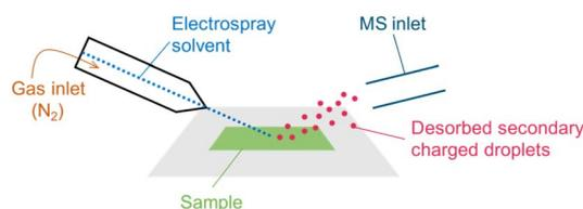
Fig. 1 Schematic representation of a DESI-MS source.
