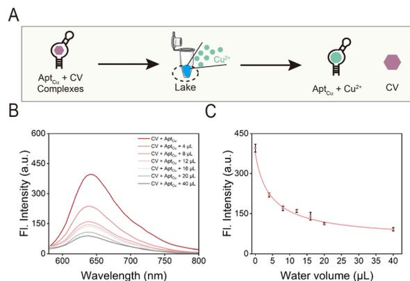
Fig. 4 (A) Schematic diagram of NIRapt-based  $\text{Cu}^{2+}$  detection in raw lake water. (B) Fluorescence emission spectra of NIRapt in the presence of varying volumes of lake water. (C) Fluorescence intensity of NIRapt when mixed with different volumes of ultrapure water or lake water samples.
