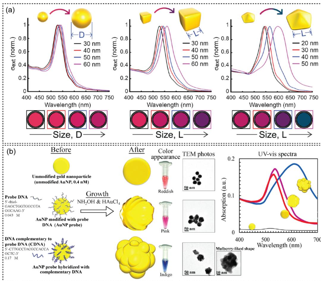
Fig. 6 (a) Calculated extinction cross-section spectra and the RGB colors derived from  $\sigma_{ext}$  of gold nanoparticles with different shapes and sizes.<sup>71</sup> (b) Schematic illustration of hybridization-mediated growth of the AuNP probe for detection of complementary DNA.<sup>72</sup>
