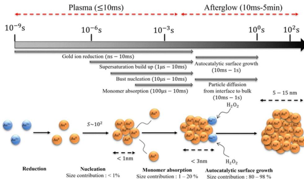
Fig. 3 Schematic of the formation mechanism of gold nanoparticles in a plasma-droplet system.<sup>48</sup>
