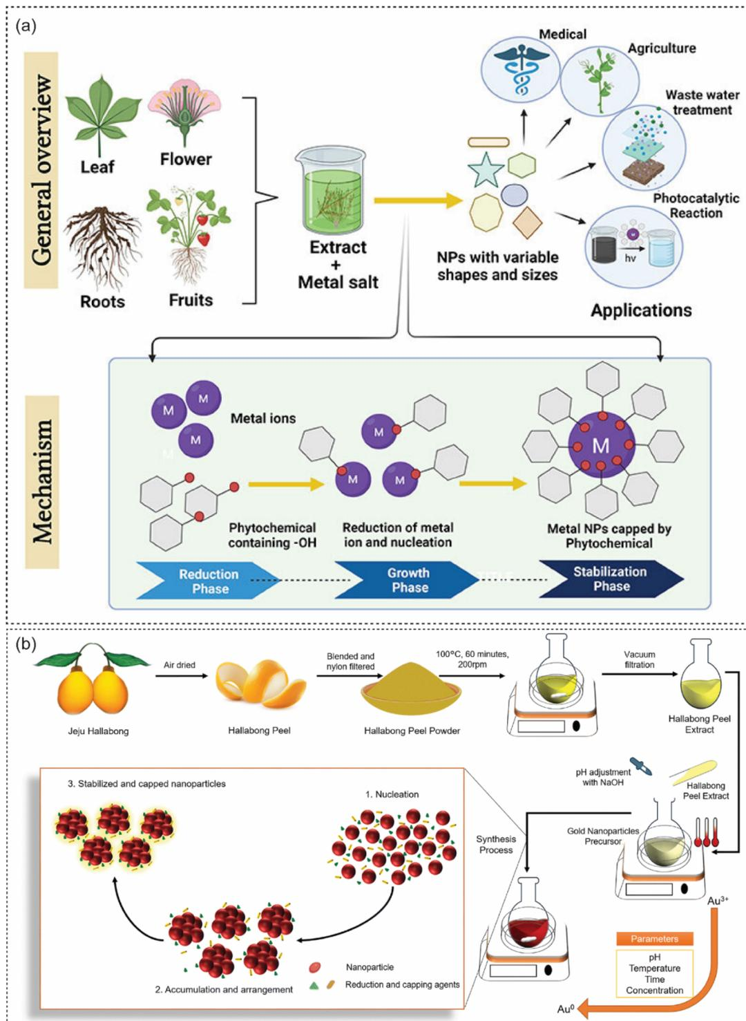
Fig. 4 (a) Schematic illustration of the general overview and mechanism involved in green synthesis of nanoparticles using extracted plants.<sup>56</sup> (b) Green synthesis of AuNPs from Jeju Hallabong extract as a reducing agent and capping agent.<sup>57</sup>
