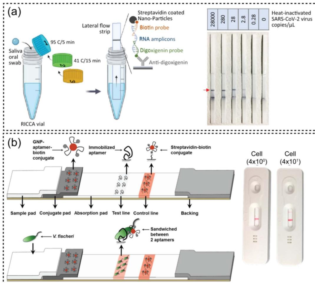
Fig. 7 (a) Direct saliva-to-RICCA-to-LF assay for the lab-free testing of SARS-CoV-2 virus.<sup>100</sup> (b) Schematic diagram of the principle for detection of the aptamer-based paper strip sensor.<sup>101</sup>
