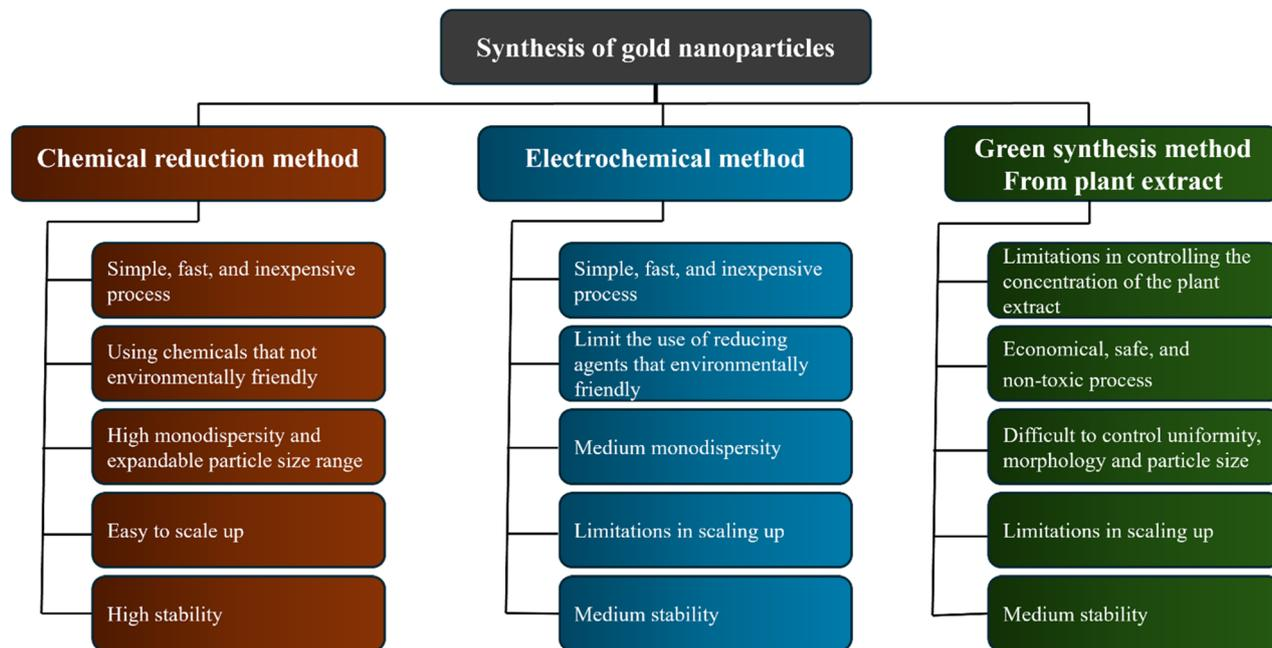
Fig. 5 Schematic summary of common features of AuNPs synthesis methods.<sup>68–70</sup>
