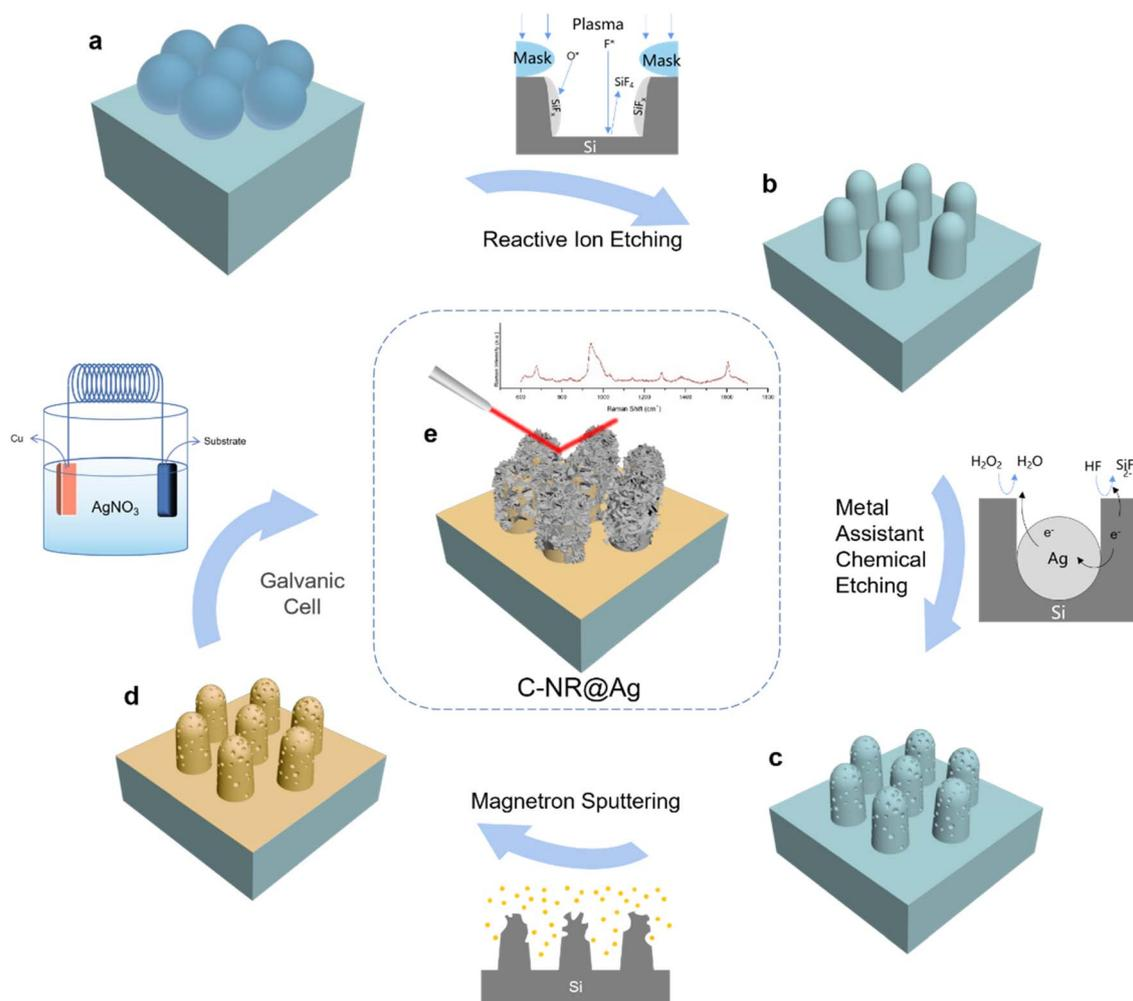
Fig. 1 Schematic of the C-NR@Ag substrate preparation process. (a) SiO<sub>2</sub> microspheres on the substrate surface; (b) the nanorod structure formed by RIE; (c) the cavity-nanorod structure formed by MACE; (d) gold film on the substrate; (e) silver plates formed by galvanic cell deposition.
