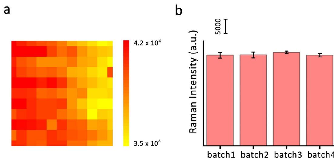
Fig. 4 (a) The uniformity of the substrate using the characteristic peak intensity of  $1078 \text{ cm}^{-1}$ . (b) The reproducibility of the substrate using the characteristic peak intensity of  $1078 \text{ cm}^{-1}$  based on the Raman spectra in Fig. S9.†
