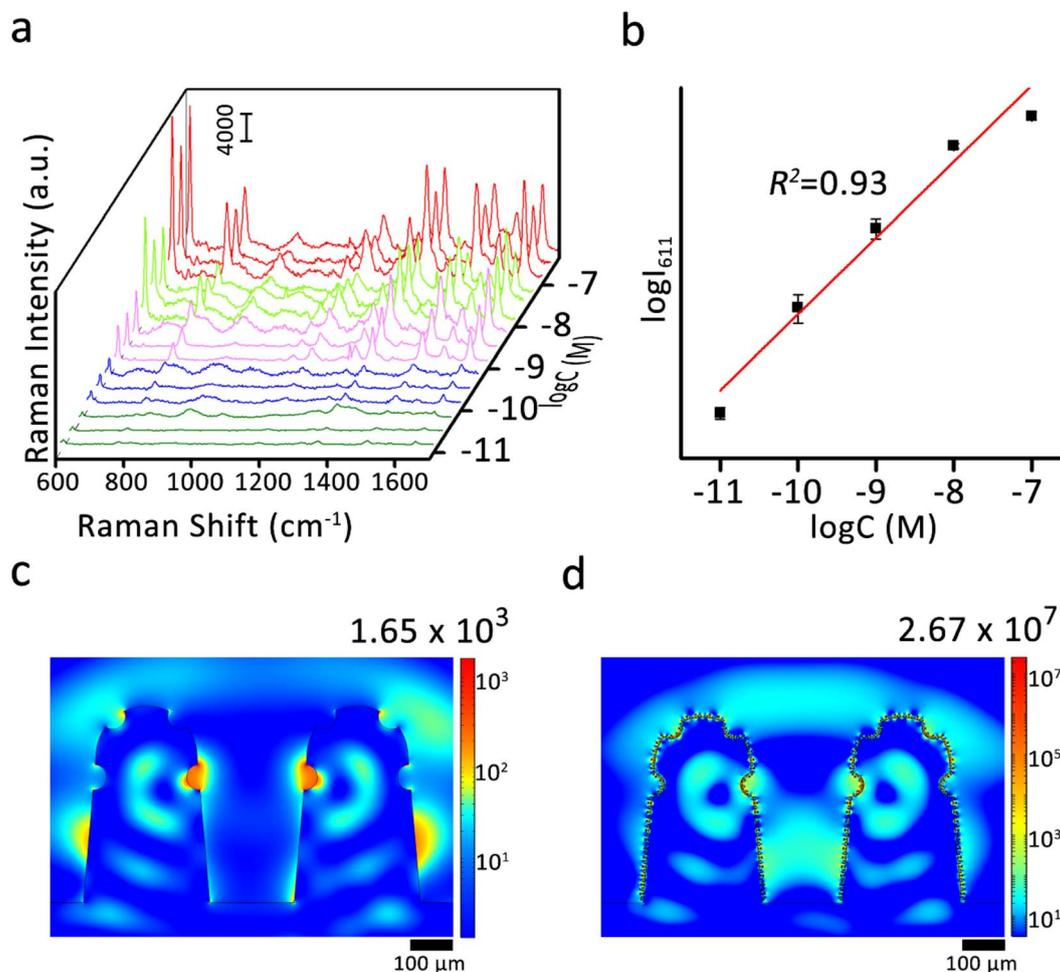
Fig. 5 (a) SERS activity of the substrate using the R6G solution with concentrations ranging from  $10^{-7}$  to  $10^{-11}$  M. (b) Correlation between the log–log plot of  $I_{611}$  and  $C_{\text{R6G}}$ . The error bar was obtained by three replicate determinations based on the Raman spectra in (a). (c) The electric field simulation of the C-NR substrate. (d) The electric field simulation of the C-NR@Ag substrate.
