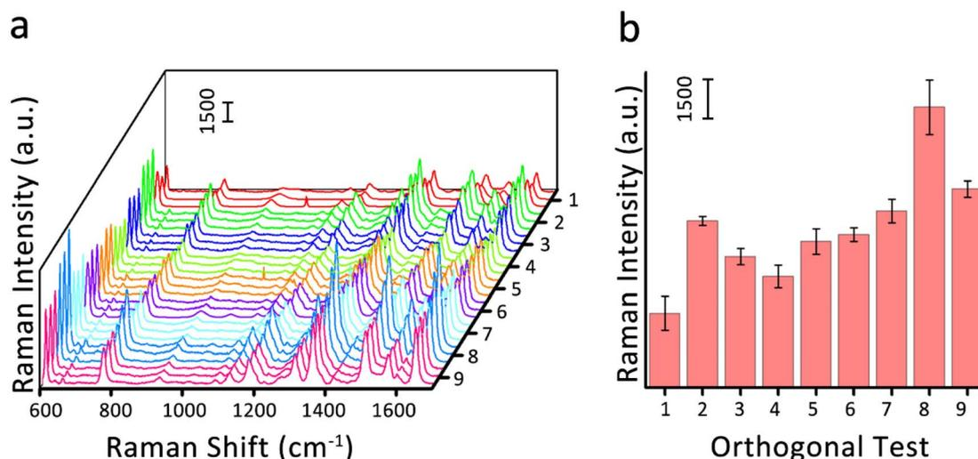
Fig. 2 (a) Raman spectra of substrates in an orthogonal test probing  $10^{-6}$  M R6G. (b) The Raman performance of substrates, using the characteristic peak intensity of  $611 \text{ cm}^{-1}$  based on (a). The error bar was calculated by three replicate determinations.
