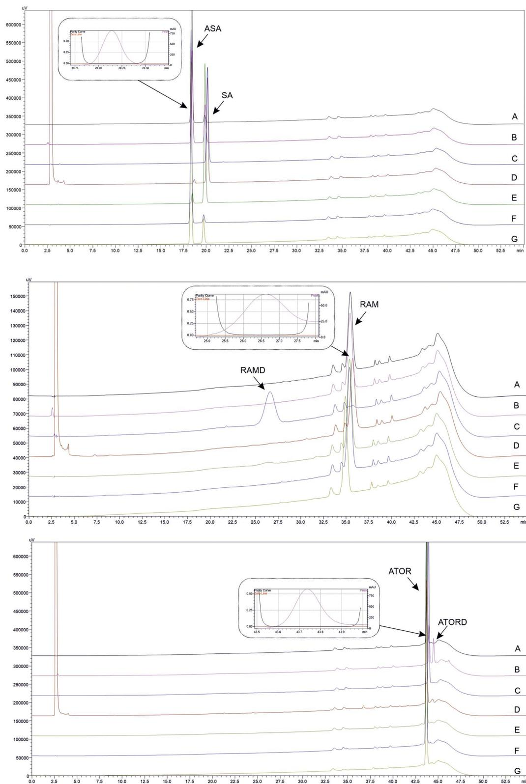
Fig. 5 Overlaid chromatograms of the analysis of (A) the standard solution of each drug ( $100 \mu\text{g mL}^{-1}$ ) and under (B) acidic, (C) alkaline, (D) oxidative, (E) thermal hydrolysis, (F) thermal degradation in the solid state, and (G) photolytic degradation stressed conditions. Insets: peak purity of each drug. For experimental conditions see the main text.
