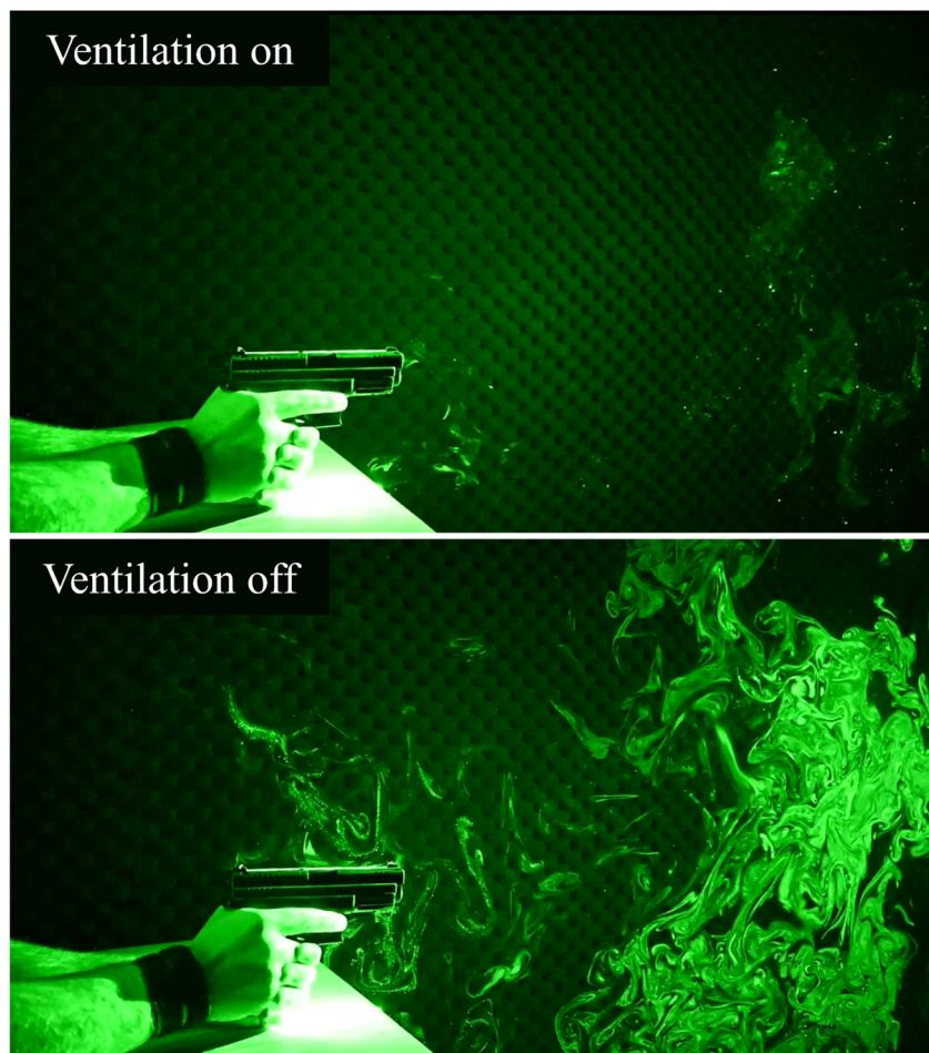
Fig. 8 Demonstration of the effects of ventilation on GSR flow. This image shows illuminated GSR particles observed in trials with the ventilation active (top) and the ventilation disabled (bottom). This image was captured five s following a single shot.
