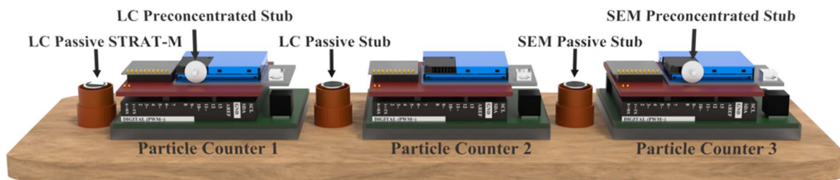
Fig. 4 Model showing the multi-method sampling device, used to carry three custom-made particle counters as well as passive collection carbon adhesive stubs and stubs affixed closely to the particle counter outlet, on which GSR that passed through the particle counters could be collected.
