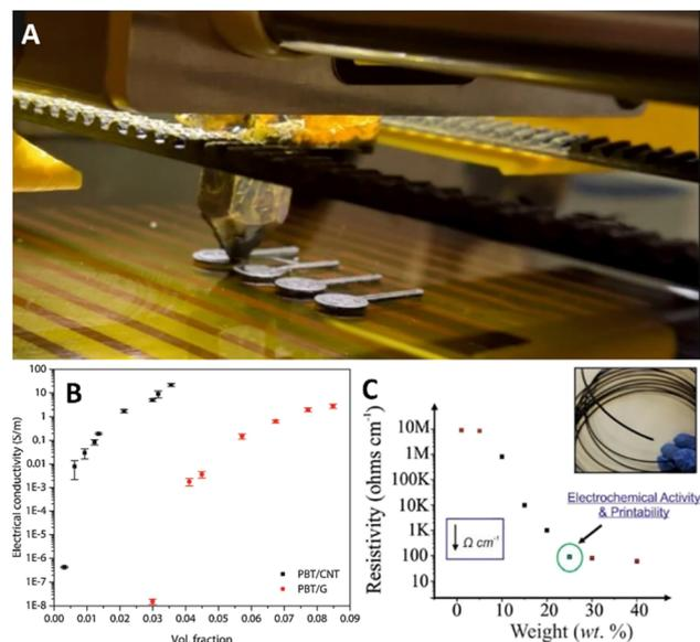
Fig. 6 (A) Fabrication of 25 wt% nanographite-loaded PLA electrode.<sup>67</sup> (B) Electrical conductivity plotted as a function of CNT and graphene volume fraction for 3D printed polymer nanocomposites.<sup>66</sup> (C) Resistivity vs. nanographite content.<sup>67</sup> Copyright, Elsevier B.V.
