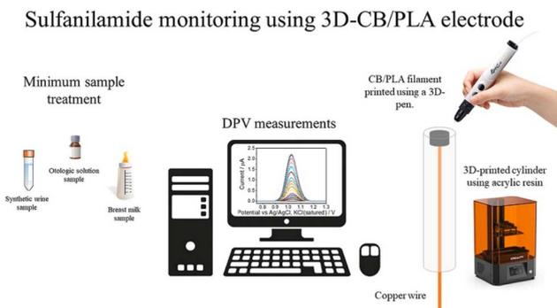
Fig. 13 3D-printed electrode for sulfanilamide monitoring.<sup>112</sup> Copyright, Elsevier B.V.
