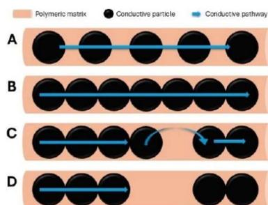
Fig. 5 Illustration of conductive networks with (A) low fraction of conductive particles, (B) the critical value, (C) small gaps, and (D) insufficient conductive material.<sup>61</sup> Copyright, MDPI.
