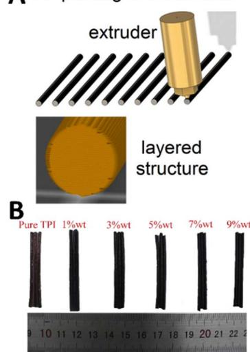
Fig. 7 (A) Geometry of PLA/CB 3D-printed electrodes. (B) Samples of pure TPI and CNTs-TPI<sub>1, 3, 5, 7, 9wt%</sub> bars.<sup>76</sup> Copyright, Elsevier B.V.
