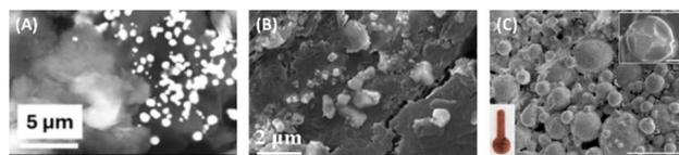
Fig. 8 SEM images of 3D printing material using (A) Au,<sup>79</sup> (B) Ag<sup>80</sup> and (C) Cu as filament.<sup>81</sup> Copyright, Elsevier B.V.
