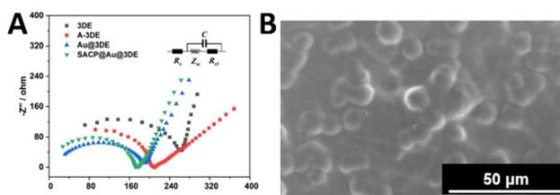
Fig. 10 (A) EIS of 3DE, A-3DE, Au@3DE and SACP@Au@3DE with frequencies between 1 and  $1 \times 10^6$  Hz. (B) SEM of prepared SACP@Au@3DE.<sup>102</sup> Copyright, Elsevier B.V.
