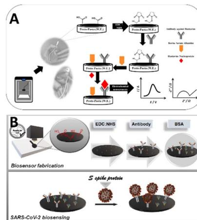
Fig. 12 Fabrication of 3D-printed electrochemical immunosensors for (A) *Listeria monocytogenes*<sup>107</sup> and (B) SARS-CoV-2 detection.<sup>37</sup> Copyright, Elsevier B.V.
