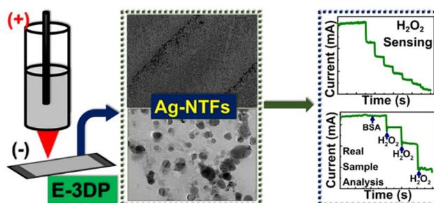
Fig. 11 Fabrication of Ag-NTF on substrates using electrochemical 3D printing for  $H_2O_2$  detection.<sup>104</sup> Copyright, American Chemical Society.
