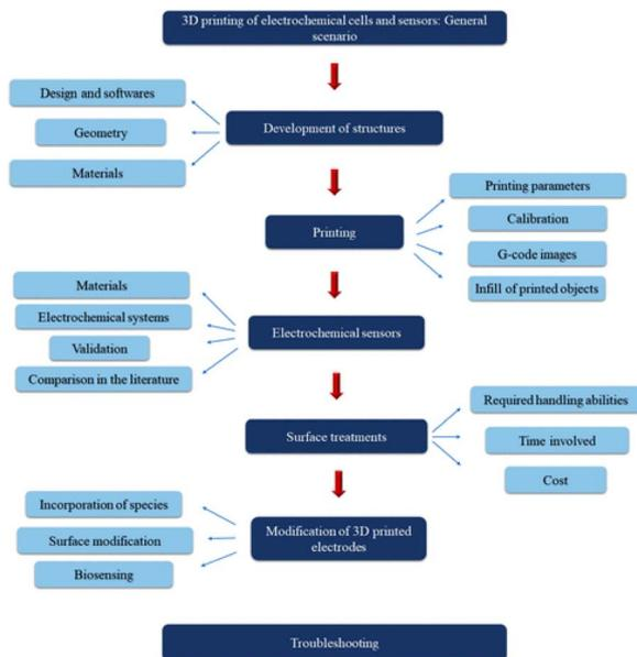
Fig. 1 Scheme of the main steps to follow in the development of 3D printing electrochemical sensors or cells.<sup>27</sup> Copyright, American Chemical Society.
