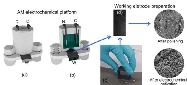
Fig. 2 Schematic representation of an efficient and commonly employed pretreatment performed on a CB/PLA 3D printed electrode.<sup>29</sup> Copyright, American Chemical Society.
