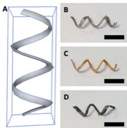
Fig. 3 Scheme of the 3D-printed helical metal electrode and photographs of 3D-printed stainless-steel electrode and after electroplating of gold and bismuth.<sup>44</sup> Copyright, American Chemical Society. Copyright, Wiley.
