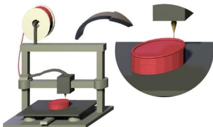
Fig. 4 Illustration of a FDM 3D printer, highlighting in the zoomed-in image the layer-by-layer deposition process, forming the final object.<sup>61</sup> Copyright, MDPI.
