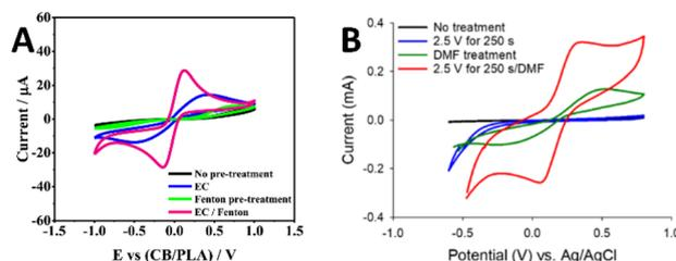
Fig. 9 (A) CVs recorded in the presence of  $[\text{Fe}(\text{CN})_6]^{4-/3-}$  using 3D printed electrodes with no pre-treatment, treated *via* electrochemical approach, Fenton process and both electrochemical/Fenton activation.<sup>96</sup> (B) CVs recorded in the presence of  $[\text{Fe}(\text{CN})_6]^{4-/3-}$  using DMF-treated 3D electrodes.<sup>97</sup> Copyright, Elsevier B.V. and American Chemical Society.
