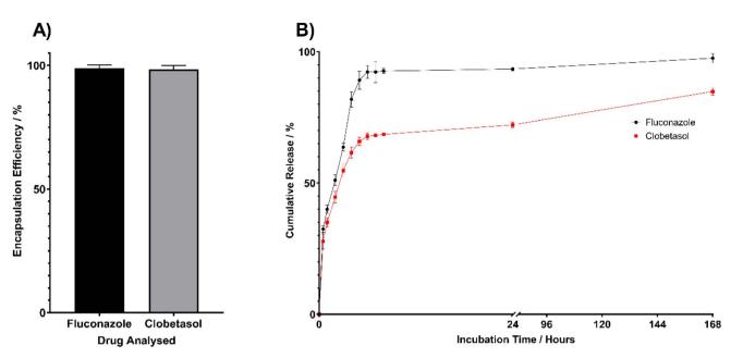
Fig. 4 (A) Mean encapsulation efficiency of FLU and CP in the PVA films used to calculate the cumulative release during the drug release study. (B) Cumulative release profile of FLU and CP from a model biomaterial, PVA hydrogel, over a 24-hour period demonstrating the potential applications of the dual detection and quantification method described here.
