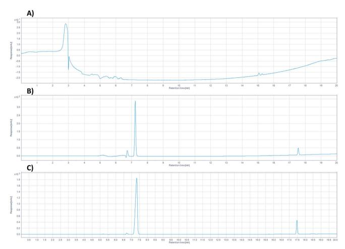
Fig. 1 Chromatograph spectrum of (A) a blank sample using the MeOH: dH<sub>2</sub>O buffer, (B) FLU-CP in a concentration of 0.25 mg per mL FLU, 5  $\mu$ g per mL CP and (C) FLU-CP in a concentration of 2.5 mg per mL FLU, 50  $\mu$ g per mL CP, respectively where the x-axis represents the time in minutes and the y-axis represents the peak height in mAU, without blank subtraction.
