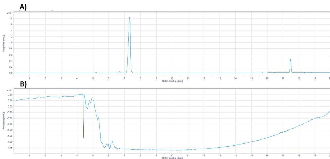
Fig. 2 Chromatograph spectra of (A) a sample of the highest sample concentration used in the calibration curve (FLU-CP at 2.5 mg mL<sup>-1</sup> and 50  $\mu\text{g mL}^{-1}$  respectively) (B) a blank sample (MeOH : dH<sub>2</sub>O buffer) injected immediately after the highest concentration sample, without blank subtraction.
