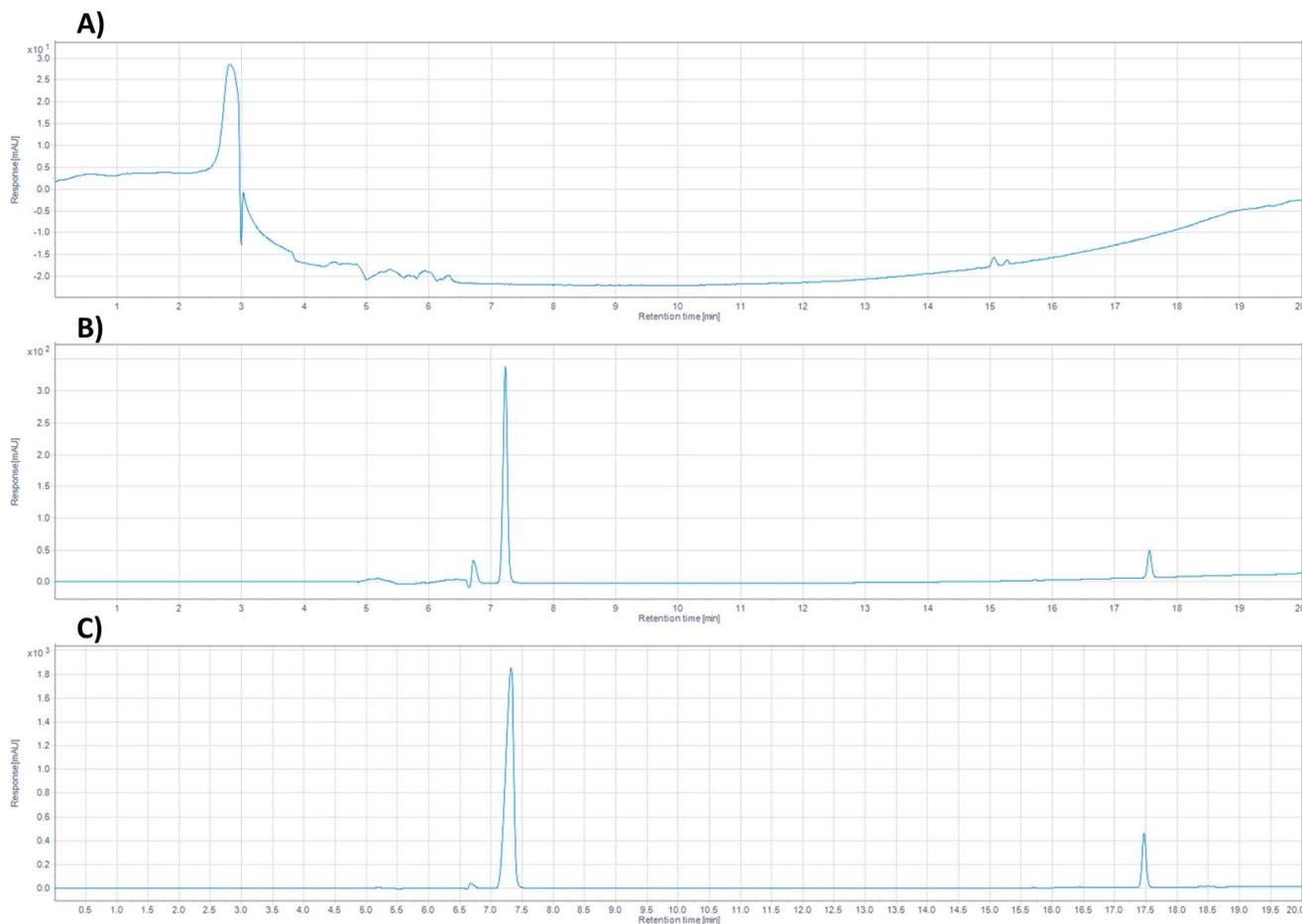
**Fig. 1** Chromatograph spectrum of (A) a blank sample using the MeOH : dH<sub>2</sub>O buffer, (B) FLU–CP in a concentration of 0.25 mg per mL FLU, 5 µg per mL CP and (C) FLU–CP in a concentration of 2.5 mg per mL FLU, 50 µg per mL CP, respectively where the x-axis represents the time in minutes and the y-axis represents the peak height in mAU, without blank subtraction.
