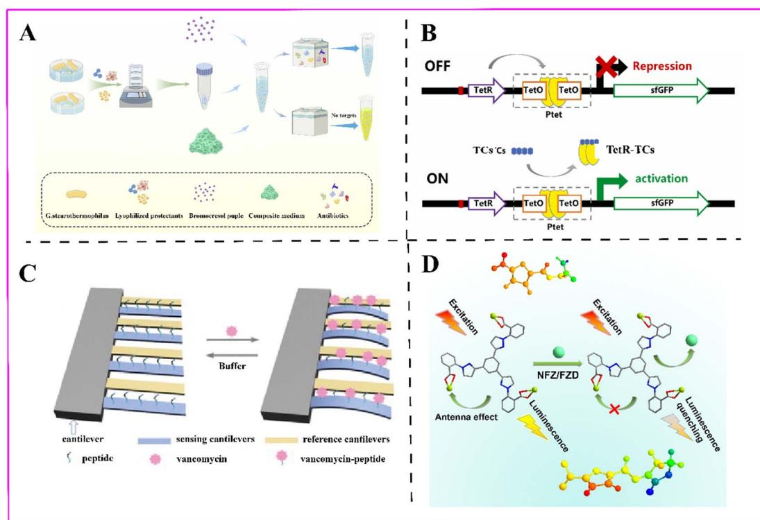
Fig. 4 Microorganism-, cell-, peptide- and MOF-based methods for antibiotic detection. (A) Multiplex platform for detecting multiple antibiotics.<sup>73</sup> (B) Basic principle of a whole cell biosensor for TC detection.<sup>74</sup> (C) Schematic illustration of reversible VAN detection.<sup>75</sup> (D) Mode of Tb-TCPB distinguishing between different types of antibiotics.<sup>76</sup>
