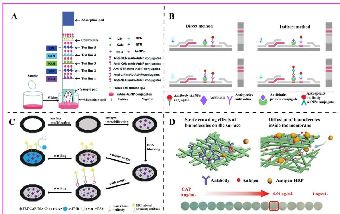
Fig. 2 Antibody-based methods for antibiotic detection. (A) Schematic of the ICA method.<sup>26</sup> (B) Direct and indirect LFIA methods.<sup>27</sup> (C) Schematic of the PAS method.<sup>28</sup> (D) Nanofiber membrane-based ELISA detection method.<sup>29</sup>
