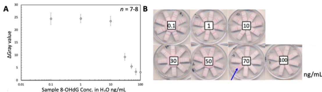
Fig. 4 (A) 8-OHdG concentration-dependent response of assays performed with device type B (8-OHdG = 0.1, 1, 10, 30, 50, 70, 100 ng mL<sup>-1</sup>), and (B) color scans of corresponding devices; error bars represent one standard deviation from the mean ( $n = 7$  or  $8$ ); blue arrow in (B) marks an LFIA lane with irregular flow behavior.
