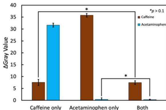
Fig. 7 Signal intensities observed for samples containing a single target ( $200 \text{ ng mL}^{-1}$  of caffeine or acetaminophen) or a mixture (caffeine =  $200 \text{ ng mL}^{-1}$  and acetaminophen =  $200 \text{ ng mL}^{-1}$ ) on LFIA device type P; error bars represent one standard deviation from the mean ( $n = 4$ ; signal acquired from 4 lanes of a single device).
