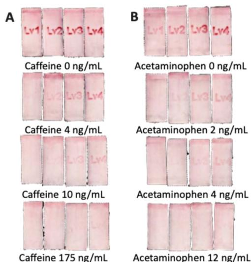
**Fig. 10** Text-displaying results for the semi-quantitative detection of (A) caffeine = 0, 4, 10, 175 ng mL<sup>-1</sup>, (B) acetaminophen = 0, 2, 4, 12 ng mL<sup>-1</sup> in artificial urine samples. The figure shows a zoom-in to each LFIA lane on a single device; brightness, contrast and saturation have been modified to improve visibility; the unmodified originals of overall devices are shown in Fig. S6.†
