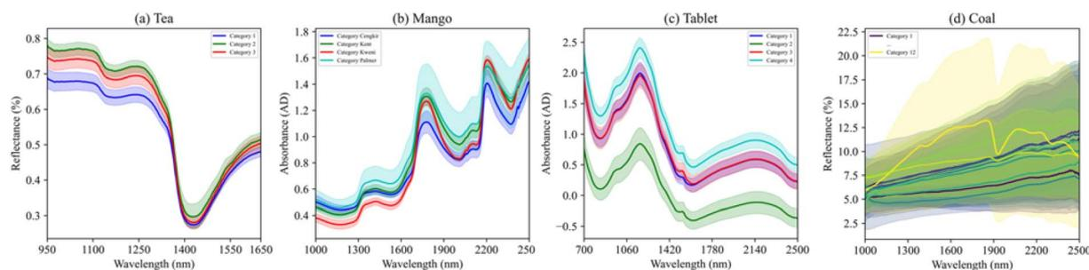
Fig. 4 Presents the raw spectra of (a) tea, (b) mangoes, (c) tablets, and (d) coal, respectively, illustrating the mean  $\pm$  standard deviation of samples from various varieties. The curves depicted are averages of the spectra, with the upper and lower boundaries of the translucent areas indicating the  $\pm$  standard deviation.
