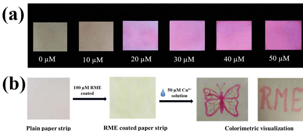
Fig. 7 (a) Colour changes of the RME sensor filter paper test strips with the increasing concentration of the Cu<sup>2+</sup> solution. (b) Colour changes observed upon the addition of Cu<sup>2+</sup> in the stock solution of the RME-soaked paper strip.
