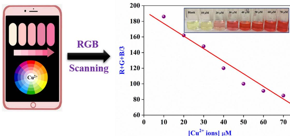
Fig. 8 The calibration curve of the RGB color response using a smartphone and the inset shows a color variance of RME with different amounts of  $\text{Cu}^{2+}$  ions in DMF/aqueous (1 : 2, v/v) medium.
