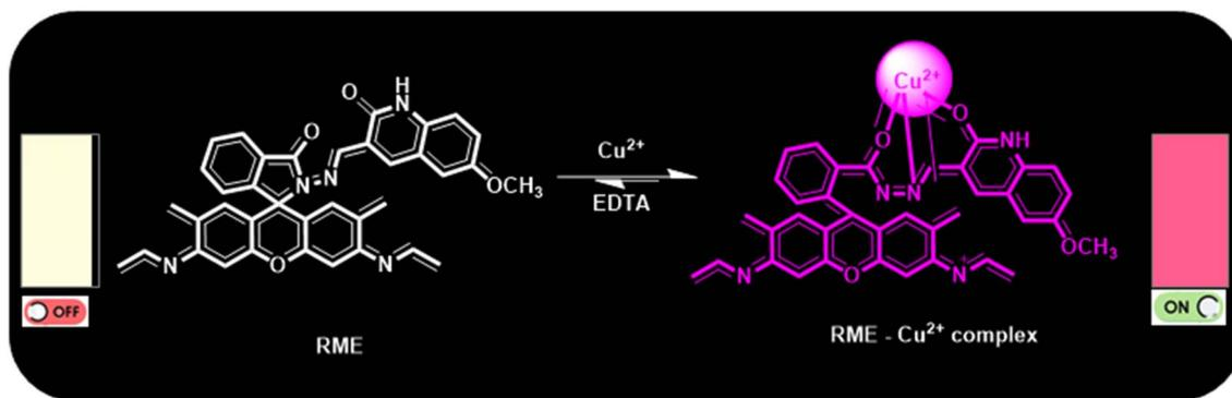
Scheme 2 Plausible mechanism for the formation of the RME–Cu<sup>2+</sup> complex and reversibility with a chelating agent, EDTA.
