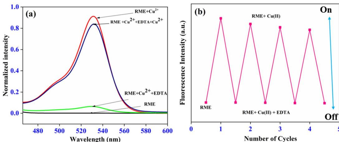
Fig. 5 Reversibility spectra (a) and cycle (b) of RME towards Cu<sup>2+</sup> (100 μM) along with EDTA (100 μM).
