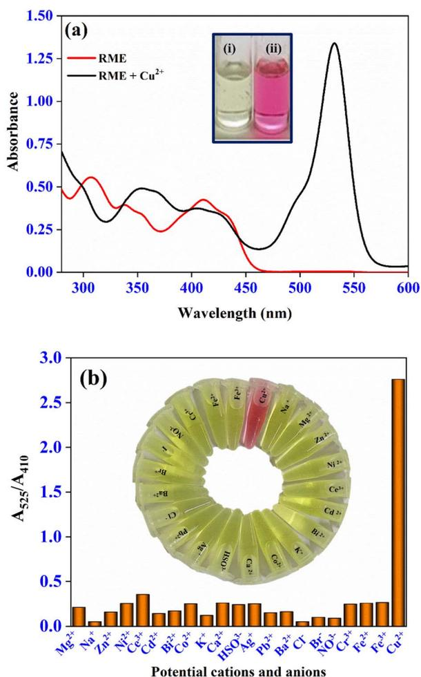
Fig. 1 UV-vis absorption spectral profile (a) for RME (10 μM) and after the addition of Cu<sup>2+</sup> ions (100 μM) and the inset represents the RME before (i) and after (ii) the addition of Cu<sup>2+</sup> ions into the receptor RME in DMF/water (1:2, v/v) medium. Bar graph (b) of RME with the addition of different metal cations and anions and the inset visualizes the notable color changes of RME solution containing different metal cations and anions in DMF/water (1:2, v/v) medium.
