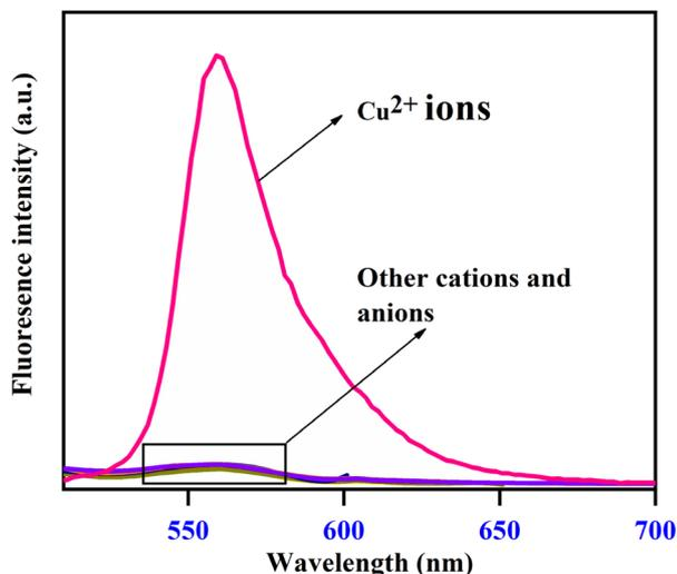
Fig. 9 Fluorescence spectra of RME with different metal cations and anions including  $Mg^{2+}$ ,  $Na^+$ ,  $Zn^{2+}$ ,  $Ni^{2+}$ ,  $Cu^{2+}$ ,  $Ce^{3+}$ ,  $Cd^{2+}$ ,  $Bi^{2+}$ ,  $K^+$ ,  $Co^{2+}$ ,  $Ca^{2+}$ ,  $Co^{2+}$ ,  $HSO_3^-$ ,  $Ag^+$ ,  $Pb^{2+}$ ,  $Cl^-$ ,  $Br^-$ ,  $Ba^{2+}$ ,  $I^-$ ,  $NO_3^-$ ,  $Cr^{3+}$  and  $Cu^{2+}$  in DMF/ $H_2O$  (1 : 2, v/v) medium.
