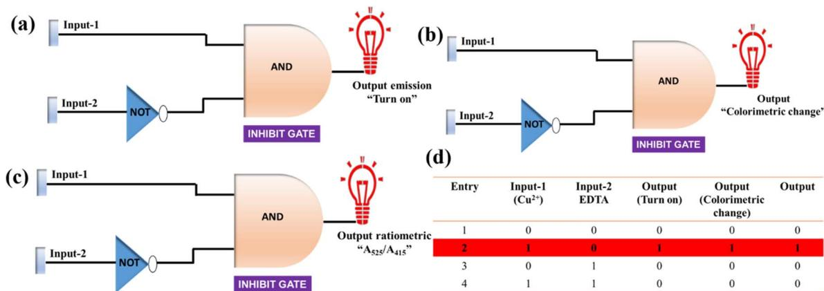
Fig. 6 (a) Construction of the truth table of the IMPLICATION logic circuit for output as emission turn on (b), output as colorimetric change (c), output as ratiometric features  $A_{525}/A_{410}$ , and the truth table (d). Truth table representation for the IMPLICATION logic gate.
