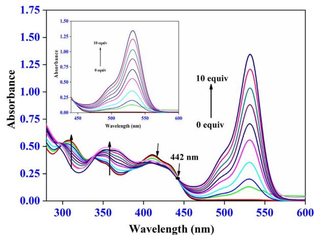
Fig. 2 UV-visible absorption spectra of RME (10 μM) upon adding Cu<sup>2+</sup> ions (0–100 μM) into DMF/aqueous (1:2, v/v) medium and the inset shows the magnified view of the newly appeared peak at 525 nm.
