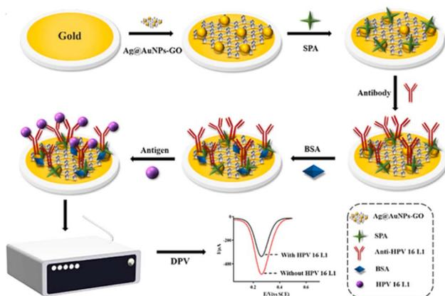
Fig. 11 Stepwise encapsulation of Ag@AuNPs-GO, SPA and anti-HPV-16 L1 antibody onto the gold electrode surface for the electrochemical detection of the target antigenic HPV-16 L1 protein.<sup>130</sup>
