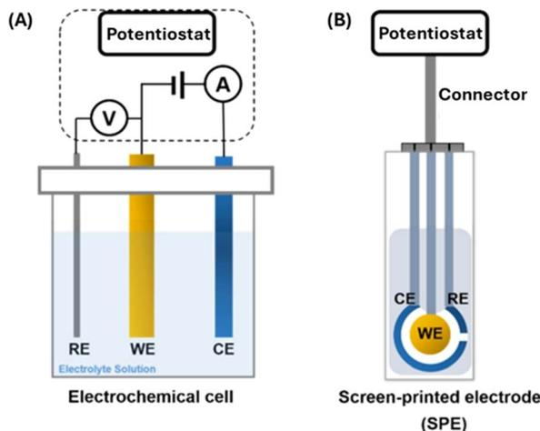
Fig. 8 Electrochemical sensors – three electrodes system (A) electrochemical cell (B) screen printed electrode (SPE).<sup>113</sup>
