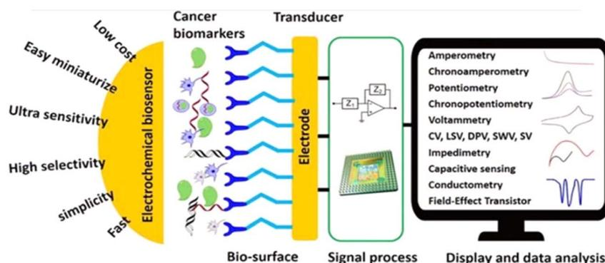
Fig. 6 Schematic diagram of advantages, component parts, and various measurement methods of electrochemical biosensor.<sup>104</sup>
