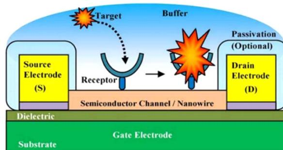
Fig. 12 Experimental illustration of a nanoscale FET biosensor.<sup>144</sup>
