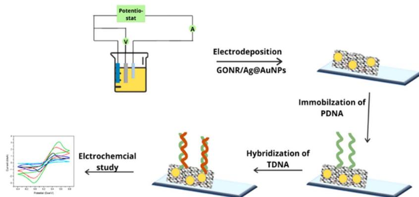
Fig. 10 Stepwise representation of the encapsulation onto the ITO surface with GONR/Ag@AuNPs and probe DNA (PDNA) for electrochemical detection of the HPV target DNA (TDNA).<sup>122</sup>
