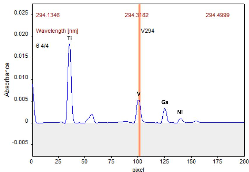
Fig. 1 Atomic lines in the same spectral window for V, Ti, Ni and Ga. Atomization peaks obtained with a solution of 15  $\mu\text{g L}^{-1}$  V, Ti, 30  $\mu\text{g L}^{-1}$  Ni and 1.5  $\mu\text{g L}^{-1}$  Ga.
