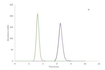
Fig. 1 (a) TDA profile for a 1% w/v G4.5 PAMAM dendrimer solution in phosphate buffer (pH 7.4) recorded at 214 nm, showing the first and second passes at windows 1 and 2. (b) TDA profile showing an overlay of three runs for a 1% w/v G4.5 PAMAM dendrimer solution in PBS (n = 3).
