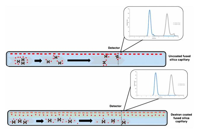
Scheme 1 Schematic representation of the charges on the capillary walls before and after dextran coating and its effect on full generation PAMAM dendrimers with respect to the Taylorgram.
