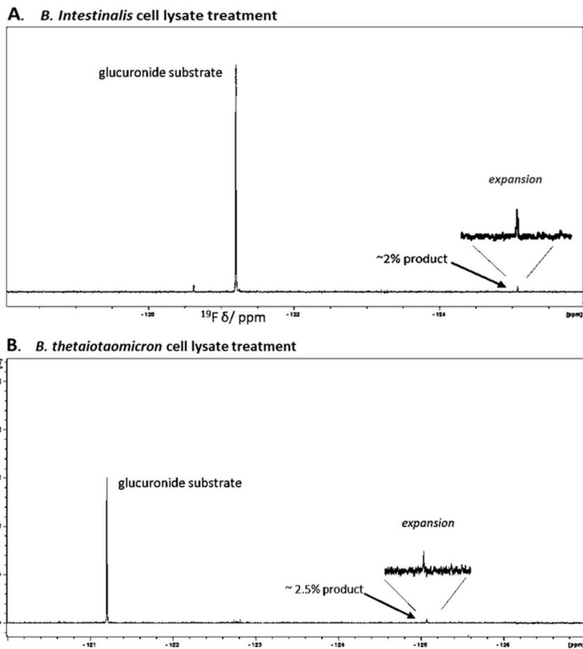
Fig. 2 Examples of limit of detection (proving signal to noise ratio of  $\sim 3$  to 1) under standard recording condition (0.1 mg substrate, 64 scans on a 600 MHz NMR instrument) employing bacterial lysates of *Bacteroides* species. (A) Hydrolysis with *B. intestinalis* lysate detected product conversion of  $\sim 2\%$  (inset). (B) Hydrolysis with *B. thetaiotaomicron* lysates detected product conversion of  $\sim 2.5\%$  (inset).
