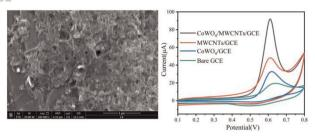
A sensitive electrochemical sensor based on CoWO<sub>4</sub>/multi-walled carbon nanotubes for the selective determination of chlorpromazine hydrochloride
