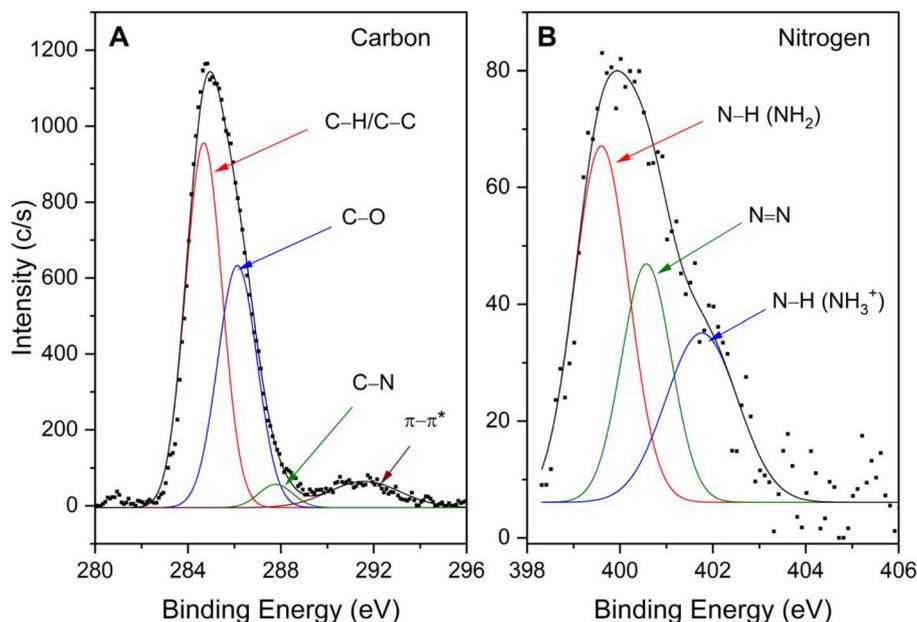
**Fig. 3** High-resolution XPS spectra and deconvoluted peaks corresponding to (A)  $\text{C}_{1s}$  and (B)  $\text{N}_{1s}$  of the *p*-PDA-derived layer on the silica particles.
