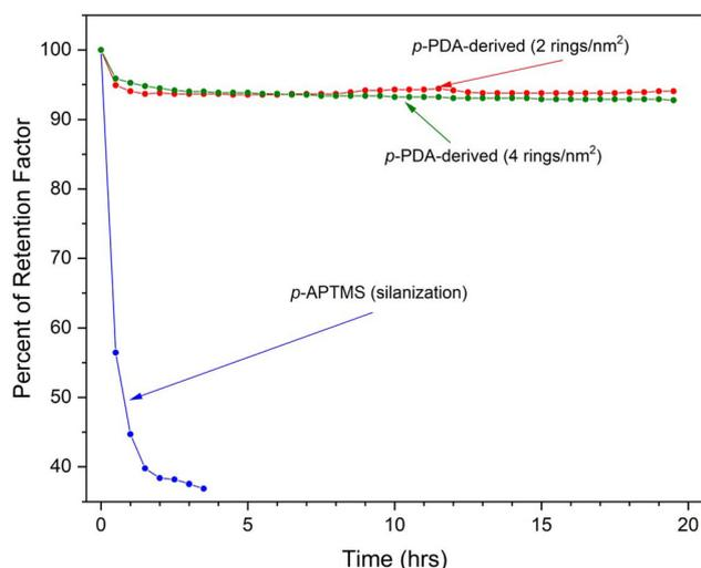
**Fig. 6** Percentage of initial retention factor as a function of time exposed to acidic conditions for three columns packed with Halo® core-shell silica particles with phases prepared by diazotization of *p*-PDA and silanization of *p*-APTMS. Test conditions: 50 : 50 water: acetonitrile with 0.5% TFA, 80 °C, flow rate of 0.2 mL min<sup>-1</sup>. Propylbenzene was used as the retention marker.
