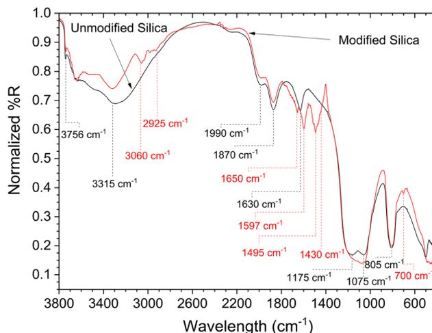
Fig. 2 DRIFTS spectra of superficially porous silica particles (Kinetex® core-shell particles) before (black trace) and after (red trace) modification with *p*-PDA *via* diazotization (4 rings per nm<sup>2</sup>).
