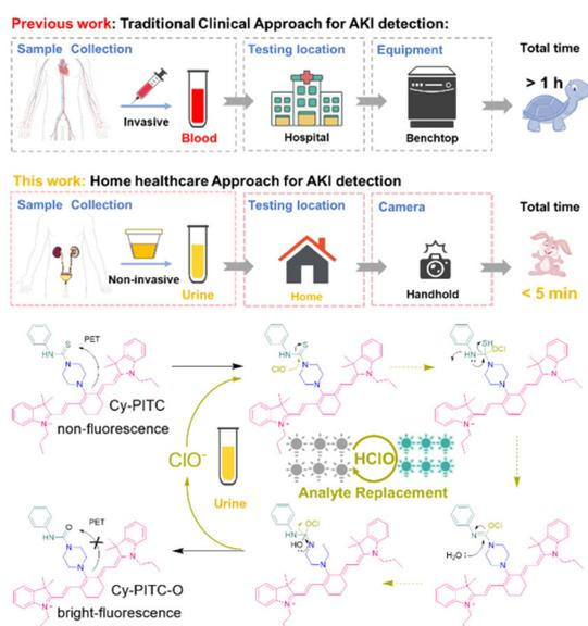
**Scheme 1** Design and advantages of Cy-PITC for non-invasive, point-of-care AKI detection. Utilizing urine samples, Cy-PITC enables non-invasive early AKI diagnosis by triggering NIR fluorescence within 5 seconds, facilitating portable home-based testing.
