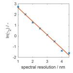
Fig. 5 The dependency of the regularisation parameter in the wavelength dimension over the spectral resolution of the analysed MW data set. The determined regularisation parameters for different spectral resolutions based on a visual inspection are shown in blue, and the fit of the logarithm of the regularisation parameter is shown in orange.
