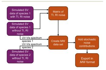
**Fig. 1** Workflow for the generation of synthetic MW SV-AUC data sets, which contain time and radial invariant noise as well as stochastic noise contributions. The steps in the purple boxes were done with SViMULATE, <sup>63</sup> all further modifications, shown in the orange boxes, were done with MATLAB.
