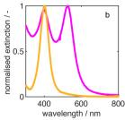
Fig. 15 Measured and normalised extinction spectra of the pure silver (yellow) and gold (magenta) nanoparticle dispersions (a) and at 310 S (yellow) and 600 S (magenta) retrieved from the 2D sedimentation coefficient distribution regularised in the sedimentation coefficient dimension (b).
