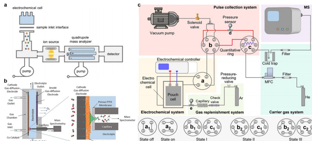
**Fig. 2** (a) Structure and composition of the DEMS setup. Reprinted with permission from ref. 33. Copyright (2024) The Royal Society of Chemistry. (b) Schematic illustration of the GDE design of flow electrolyzer MS. Reprinted with permission from ref. 37. Copyright (2021) Wiley-VCH. (c) Design and construction of the *operando* pulse EC-MS (p-EC-MS) system. Reprinted with permission from ref. 41. Copyright (2024) American Chemical Society.
