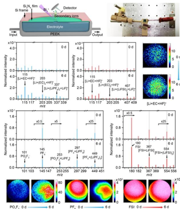
Fig. 12 Schematic illustration and photograph of the assembly of the ultrahigh-vacuum compatible microfluidic device, and representative *in situ* liquid ToF-SIMS spectra in the positive and negative ion modes of the LiPF<sub>6</sub>- and LiFSI-based electrolytes before and after high-temperature calendar aging for 6 d (144 h), highlighting the signals of ions related to hydrolysis and showing their intensity evolution. Reprinted with permission from ref. 119. Copyright (2025) Wiley-VCH.
